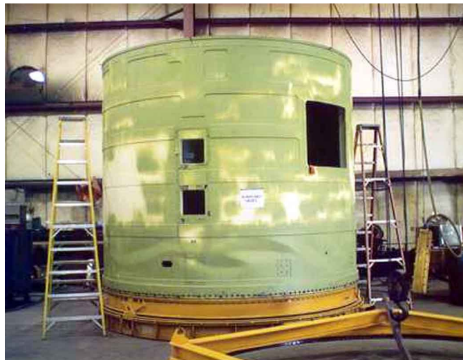
Figure 1. S/N 20022 buckled forward skirt.
