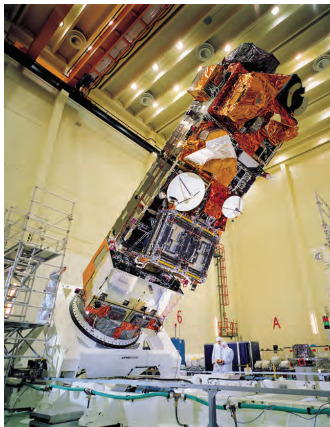
Figure 3. ENVISAT during assembly and test. Note the personnel below the satellite for scale (image from European Space Agency/A. Van Der Geest).
