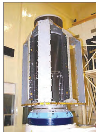
RISAT-1 main structure (image from ISRO, used with permission).
