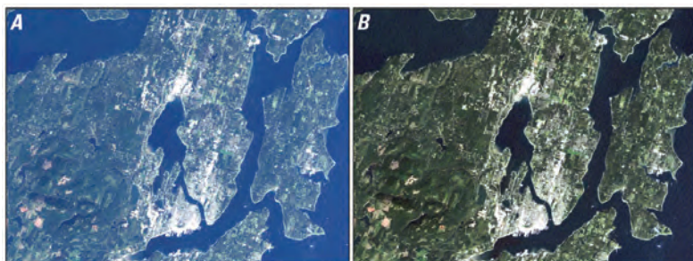
Figure 6. Landsat 5 Collection 2 images. A, top of atmosphere reflectance image (bands 4, 3, 2); B, atmospherically corrected surface reflectance image for an area over Bremerton, Washington, path 47, row 27 acquired on October 6, 2010 (images from Michelle A. Bouchard, U.S. Geological Survey).
