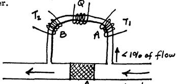
C-porous plug, laminar element
