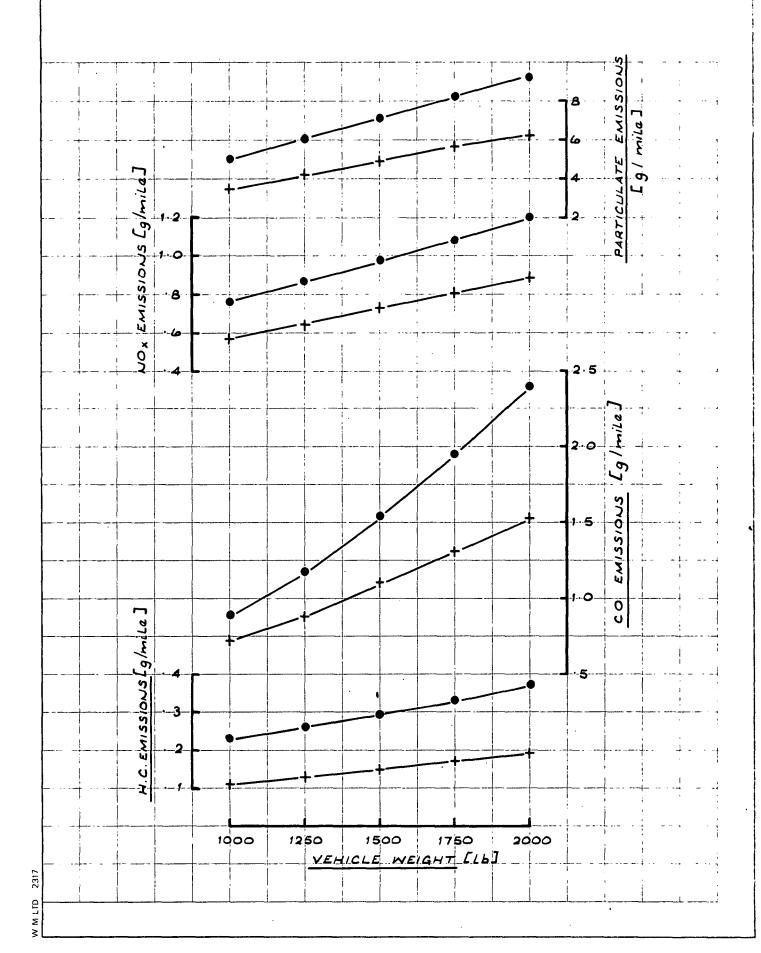
C.R.M. / W.R. FIG. No. 3 RIARDO Drg. No. D44493 PREDICTED VEHICLE PERFORMANCE CHARACTERISTICS Date 26-5-81 O.B LITRE IDI ENGINE LITRE DI ENGINE 4 [URBAN] RESULTS HIGHWAY RESULTS 100 -80 -60 mile 1h ACCELERATION TIME [Sacs] -35 30 20 20. VEHICLE WEIGHT [Lb] 1250 2000 1000 2317
