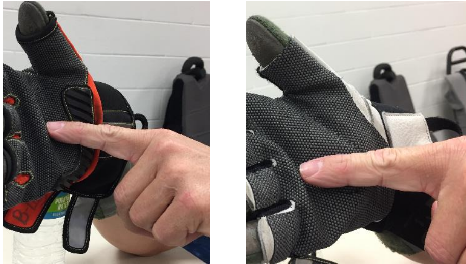
Figure 3-2 Bunched Fabric in Glove B (Left) and Glove C (Right)
