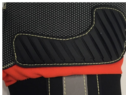
Figure 1-2 Close-up of the rubber heel on Glove B.
