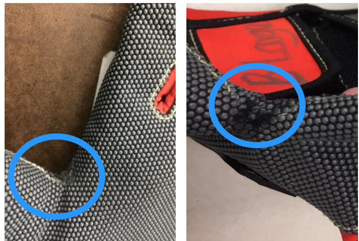
Figure 3-9 Varied Levels of Wear in the Purlicue of Glove B
