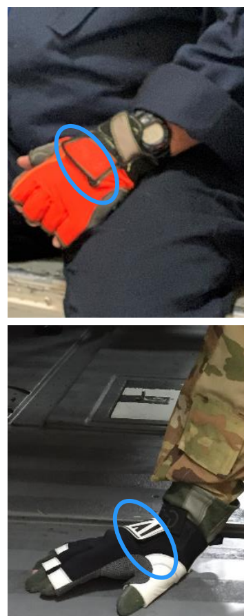
Figure 3-1 Length of Glove Cuffs B (Top) and Glove C (Bottom)
