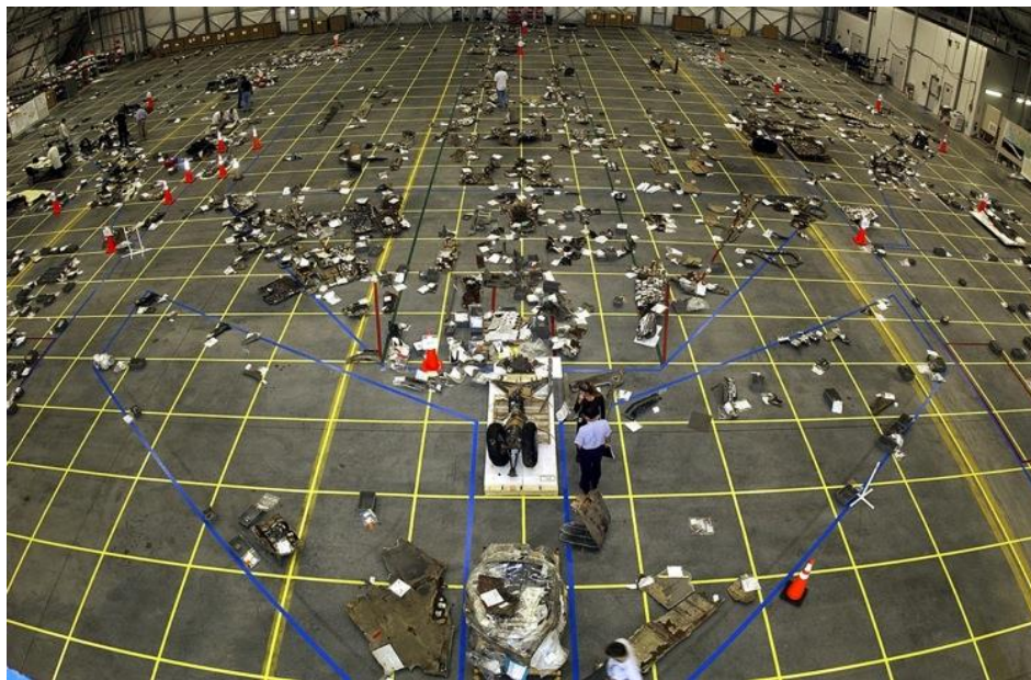
Figure 2-8. Recovered Columbia debris after break-up during re-entry. (CAIB photo by NASA, March 18, 2003, in reference 19).
