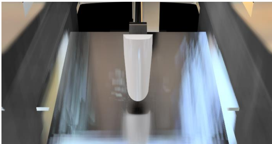
Figure 3-7. Top-view rendering of 0.50 in-radius test article at 0^\circ AoA.
