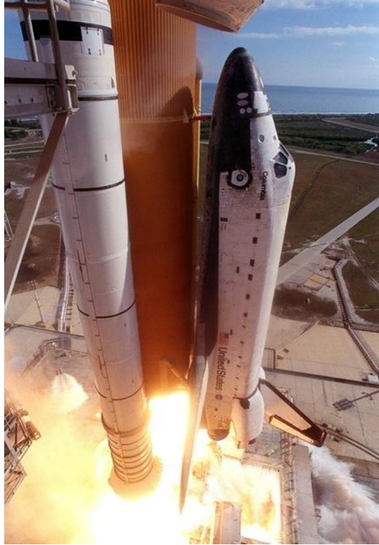
Figure 2-6. KSC Launch of Columbia STS 107. Reinforced carbon/carbon protects the wing leading edges on this vehicle. (CAIB photo by NASA, January 16, 2003, in reference 17).
