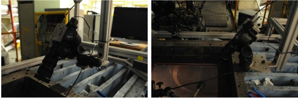
Figure 3-26. Hitachi camera aimed at the leading edge of the oil-flow test articles through the top window.
