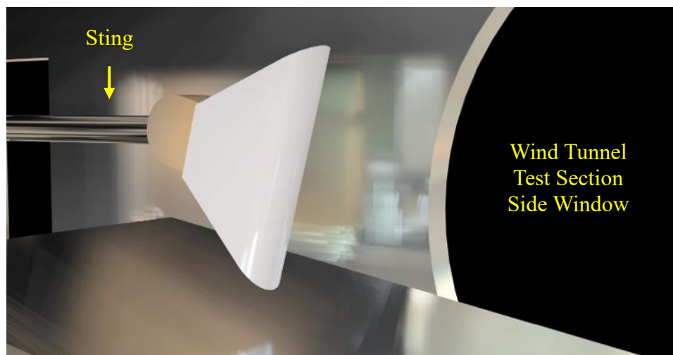
Figure 3-5. Side-view rendering of 0.50 in-radius test article at -15° AoA.
