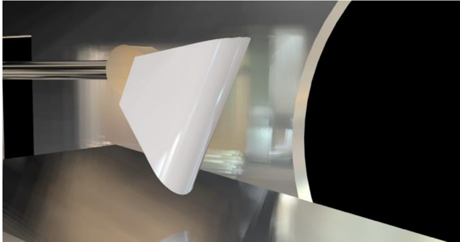
Figure 3-6. Side-view rendering of 0.75 in-radius test article at -25^\circ AoA.
