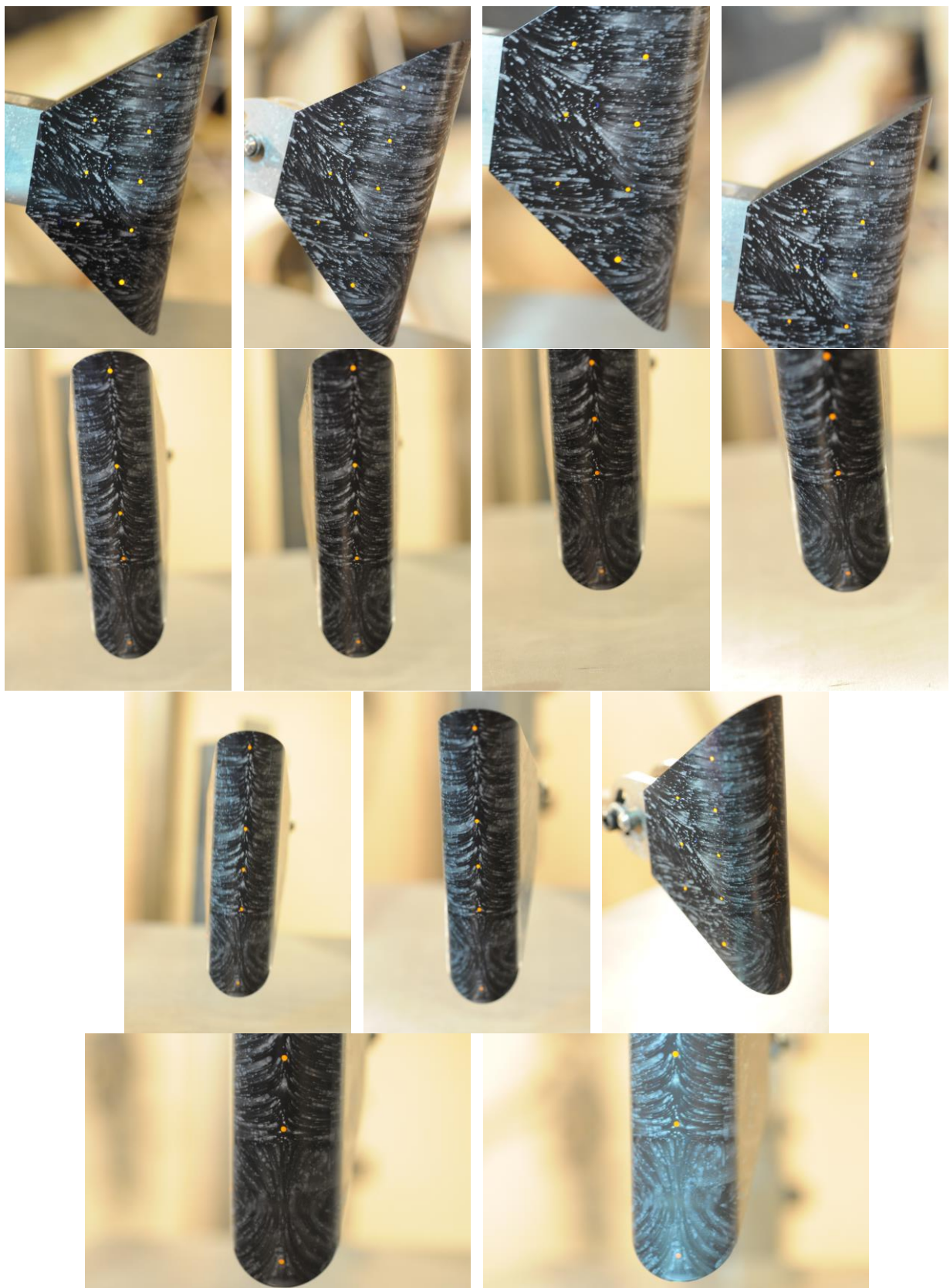
Figure D-5. Oil flow images from run 5 for the 0.50 in-radius test article at a -15^\circ AoA.
