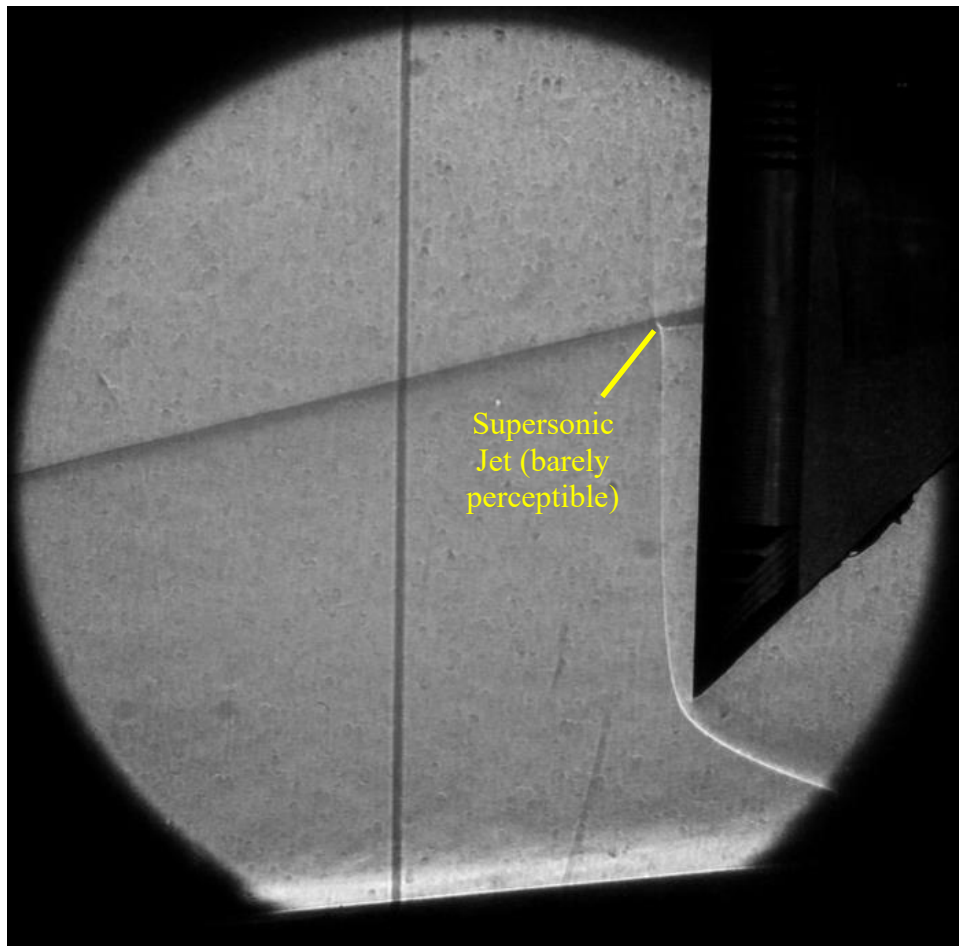
Figure 5-32. Zoom schlieren image of the Upilex® test article at a 0^\circ AoA with a 6^\circ SG angle (recolored with saturation: 0%; brightness: +40%; contrast: +20%).
