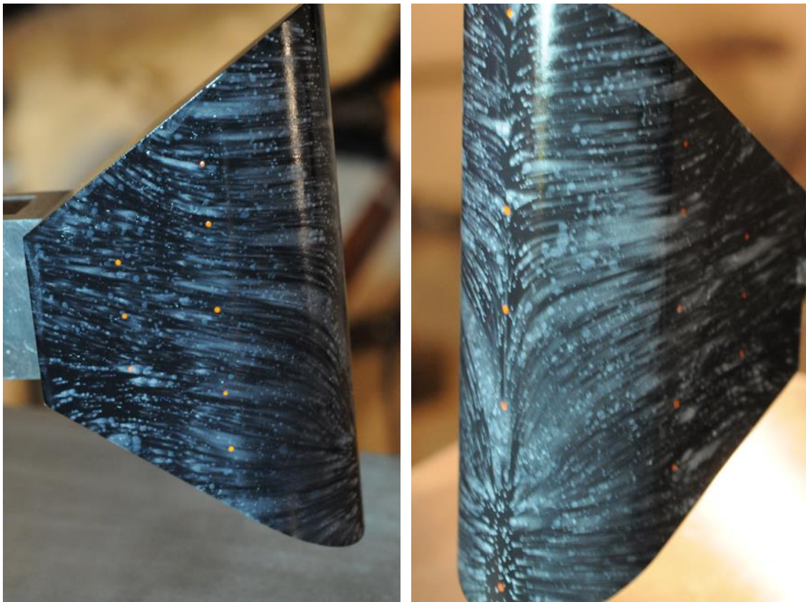
Figure 5-15. Side oil-flow images for the 0.75 in-radius metal test article at a 0^\circ AoA (both images display streamlines produced with the oil flow dots technique).
