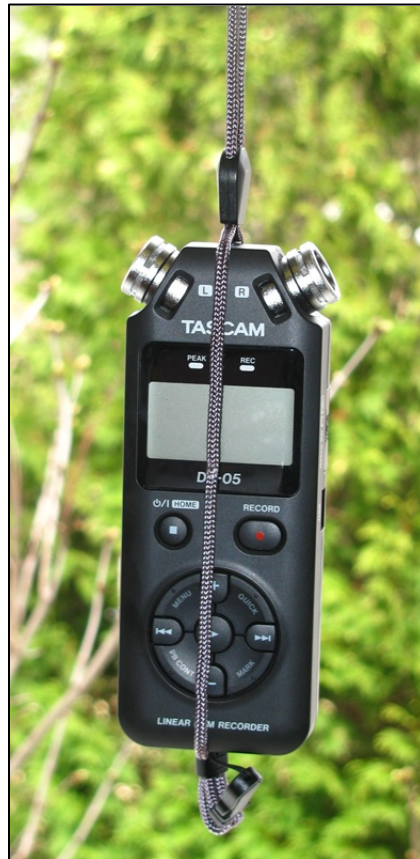
Figure S6.3. Method for hanging recorder with microphones facing up.
