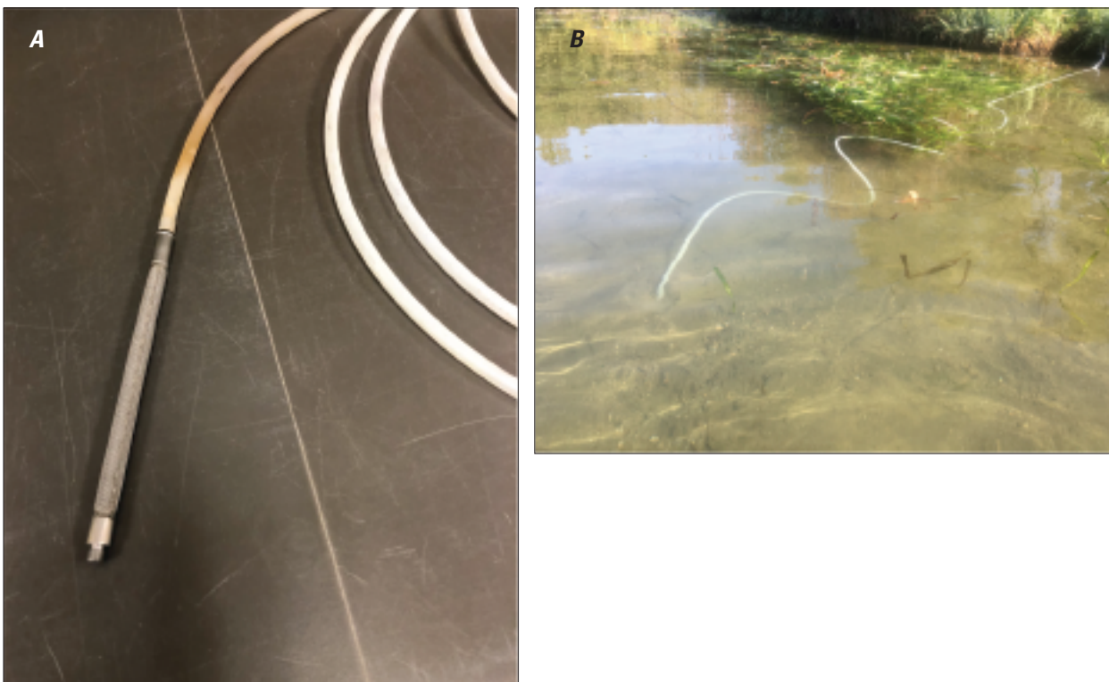
Figure 4. Components and installation of sampler used to collect shallow nearshore groundwater, Lake Spokane, Spokane, Washington. (A) Polypropylene tubing with stainless steel sample tip. (B) Final installation of the sample tip in the lakebed with sample tubing sticking out of the lakebed and towards the shore for pumping. All photos taken by Rich Sheibley, U.S. Geological Survey.
