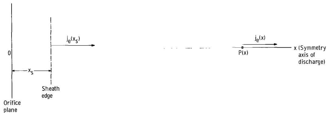
Figure 15. - One-dimensional representation of fast-electron flow density along discharge axis.
