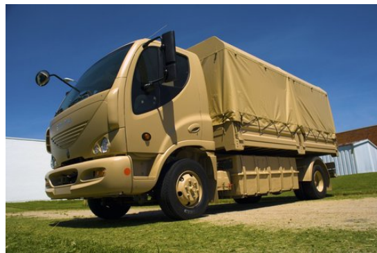
Figure A-2. The Smith Electric Newton all-electric truck, upfitted into one of many different configurable options (Credit: Smith Electric Vehicles, PIX 17631)
