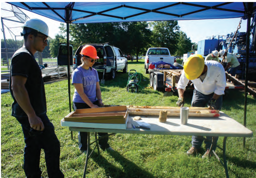
Figure 9. Photograph of a U.S. Geological Survey and Federal Highway Administration researchers observing and describing increments of sediment from a core sample at the Grist Mill drilling location in Alexandria, Va. Photograph by Jessica DeWitt, U.S. Geological Survey.
