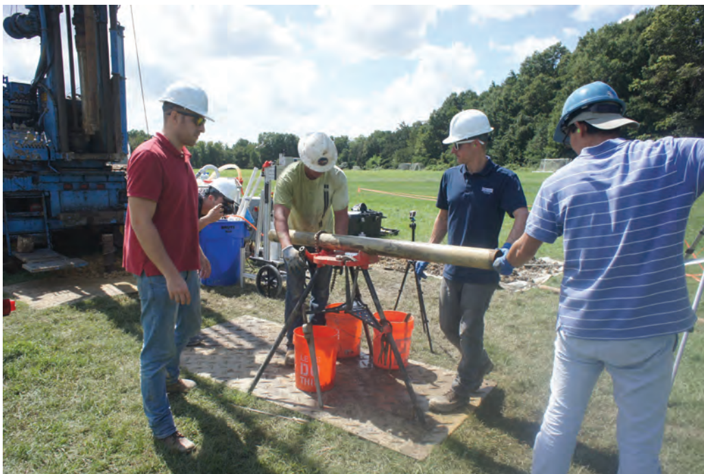
Figure 8. Photograph of a U.S. Geological Survey drill rig operator and Federal Highway Administration researchers opening the auger spoon to observe sediment from a core at the Grist Mill drilling location in Alexandria, Va. Photograph by Peter Chirico, U.S. Geological Survey.
