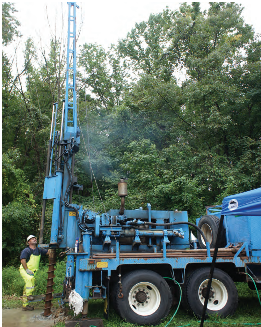
Figure 7. Photograph of a U.S. Geological Survey drill rig operator extracting a 5-ft increment of a continuous sediment core at the Huntley Meadows drilling location in Alexandria, Va. Photograph by Jessica DeWitt, U.S. Geological Survey.
