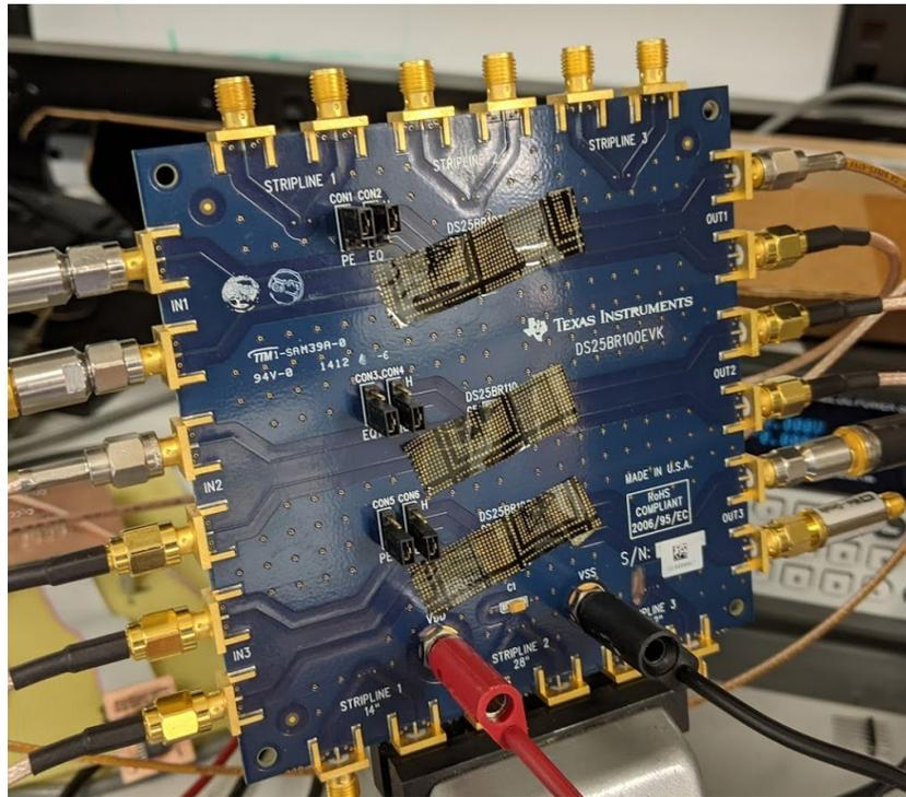
Fig. 2. DS25BR100EVK board with three decapsulated devices ready for testing.
