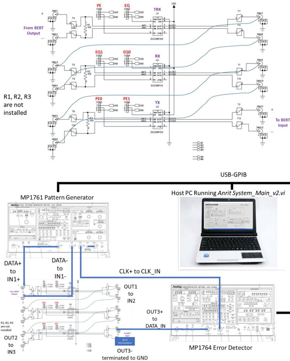
Fig. 3. Schematic of evaluation board (top) and test equipment setup (bottom).
