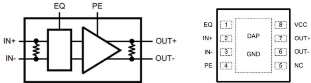
Fig. 1. Device functional diagram [DS25BR100 datasheet] and package pinout
