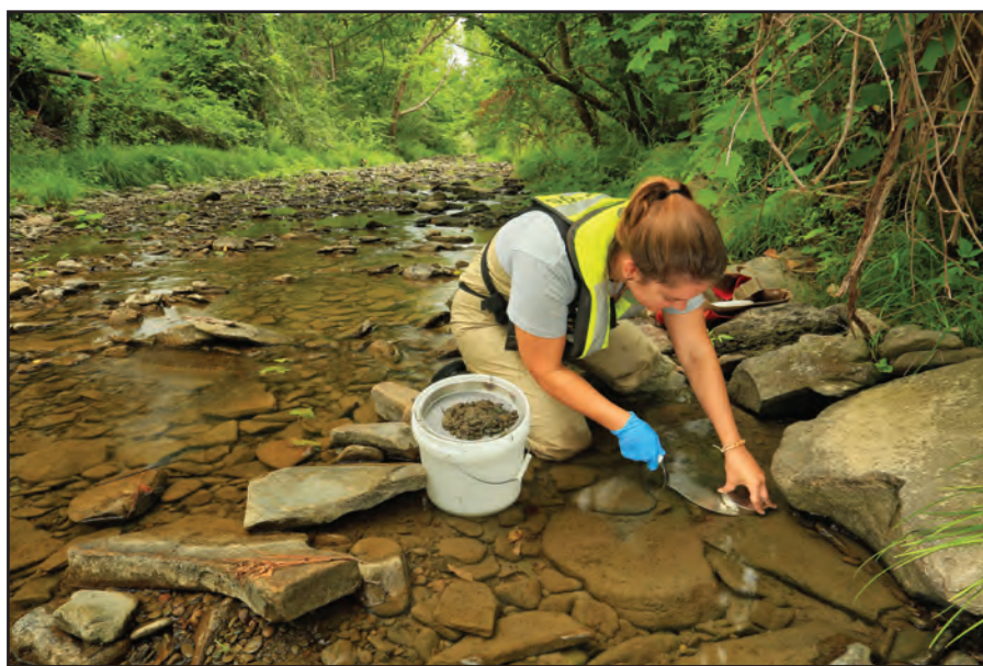
Figure 10. Collection of composite bed-sediment samples from a depositional area along a reach. Photograph by Alan Cressler, U.S. Geological Survey.
