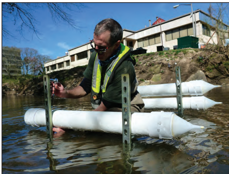
Figure 8. Installation of time-integrating suspended-sediment passive samplers by U.S. Geological Survey personnel. Photograph by Celeste Journey, U.S. Geological Survey.
