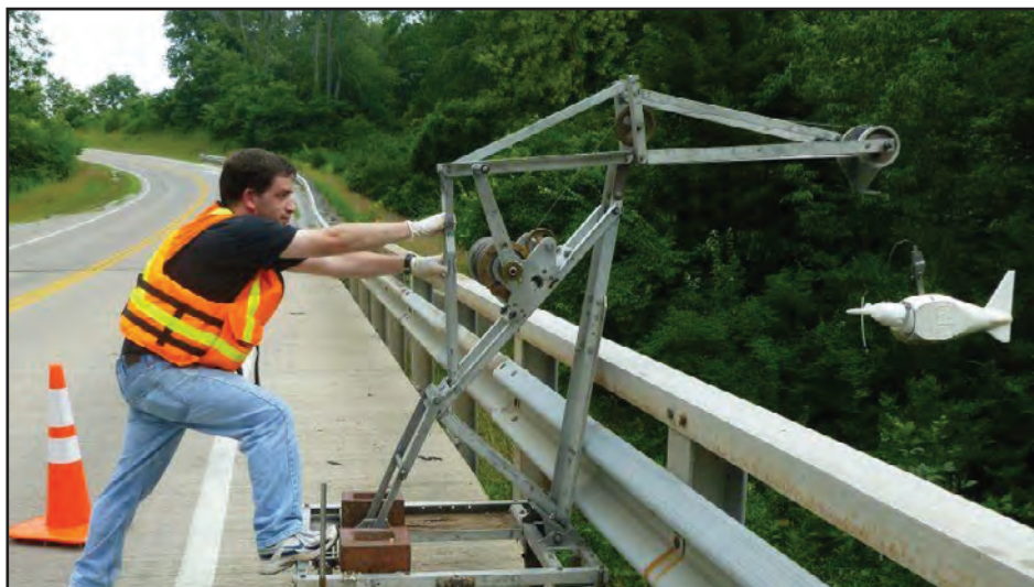
Figure 5. A hydrologist moves an isokinetic sampler into position. Photograph by Stephanie Kula, U.S. Geological Survey.
