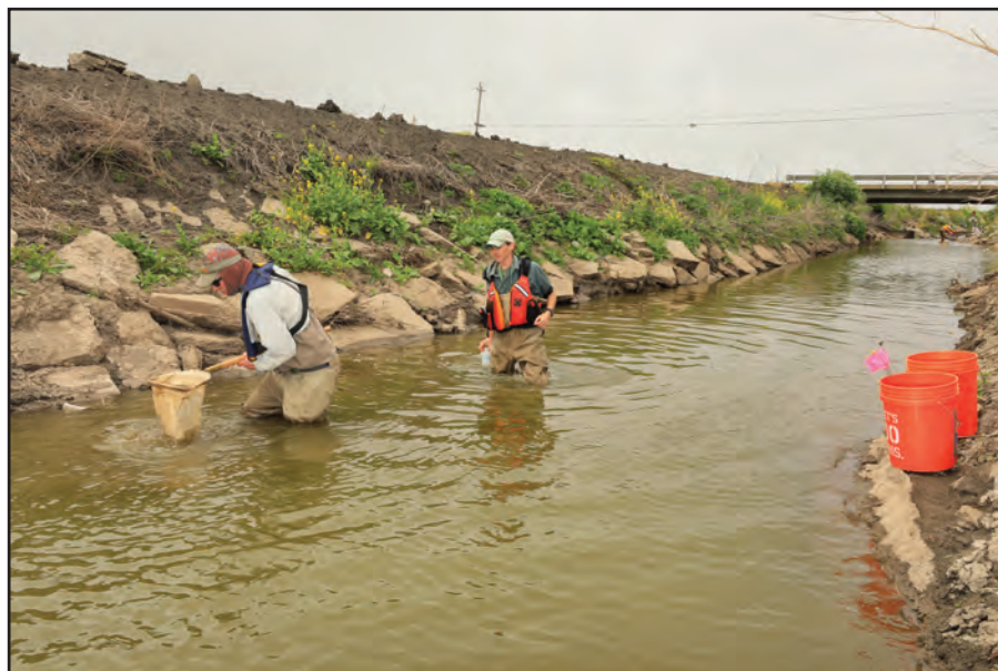
Figure 9. Invertebrate sampling with a D-frame dip net by U.S. Geological Survey personnel. Photograph by Alan Cressler, U.S. Geological Survey.
