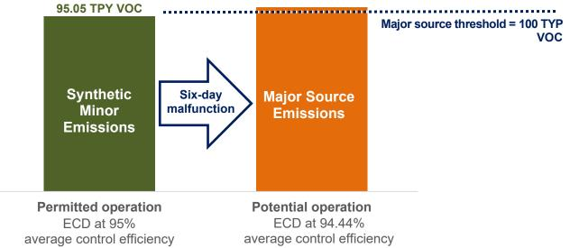
Source: OIG analysis of potential VOC emission increases due to a short-term ECD malfunction. (EPA OIG image)
