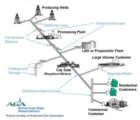
Figure D-1: Natural gas industry from production to distribution
