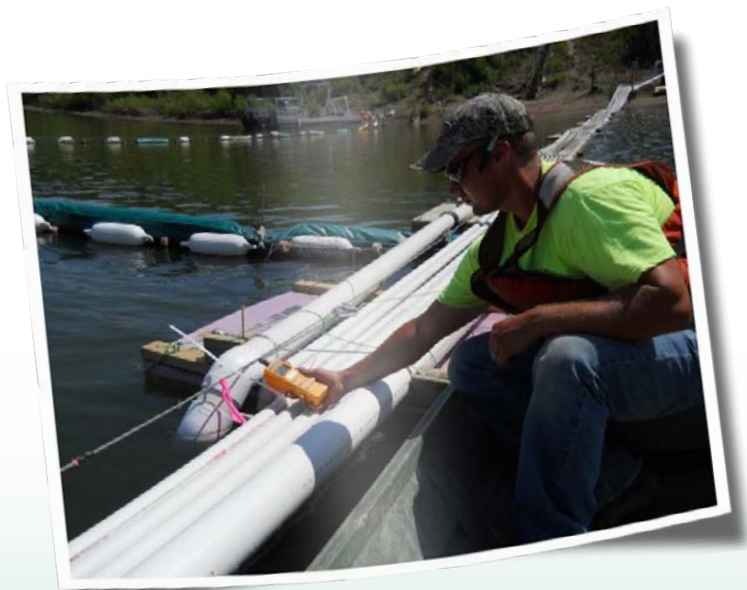
Field testing of the deployment of a carbon dioxide infusion system as a chemosensory deterrent to invasive carps in Morris, Illinois. Photograph by the U.S. Geological Survey.
