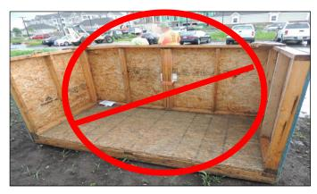
A typical job-made box consists of a wooden (e.g. plywood) platform with three walls. In this example, the job-made box was attached to a powered industrial truck (PIT) using a strap looped around the center of the wood beams that make up the longest wall and a galvanized hook. A worker was injured when the hook's safety latch failed and the platform fell to the ground.
