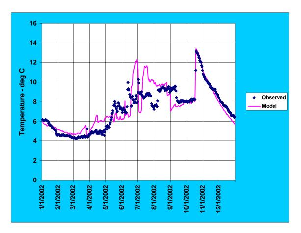
Figure 14. Simulated and observed outlet temperatures at Dworshak Dam during 2002.
