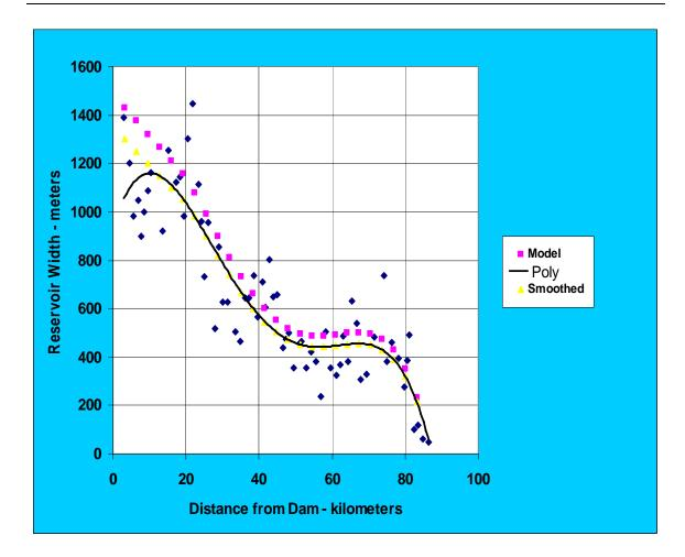
Figure 6. Measured and modeled reservoir widths of Dworshak Reservoir
