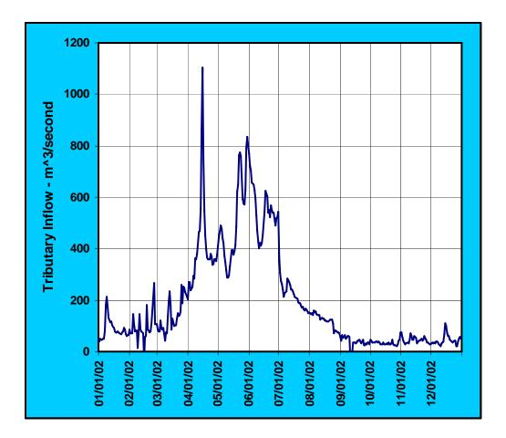
Figure 11. Tributary inflows to Dworshak Reservoir during the calendar year 2002 based on data from USGS gage station 13340600.
