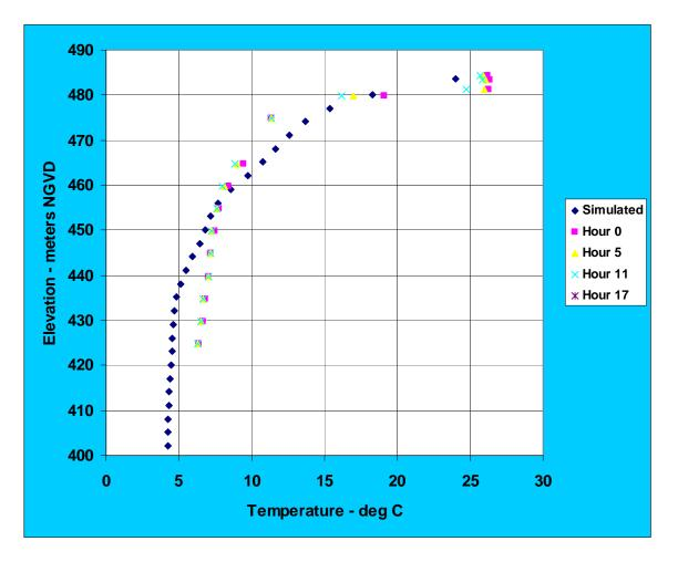
Figure 16. Simulated and observed water temperatures in Dworshak Reservoir at Dworshak Dam on July 20, 2002
