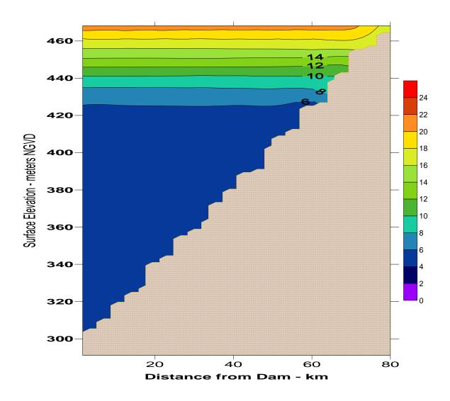
Figure 22. Simulated longitudinal temperature profiles in Dworshak Reservoir on August 28, 2002.
