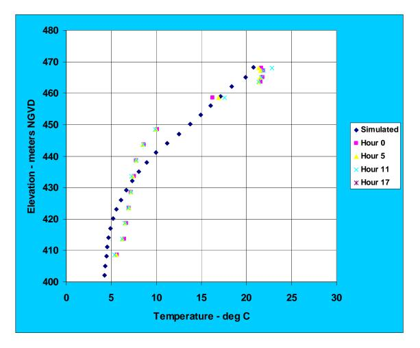
Figure 18. Simulated and observed water temperatures in Dworshak Reservoir at Dworshak Dam on August 28, 2003
