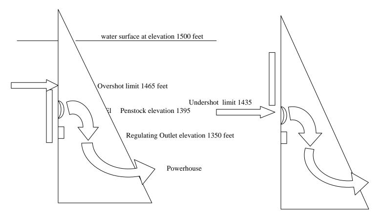
Figure 3. Dworshak Dam selective withdrawal structure schematic
