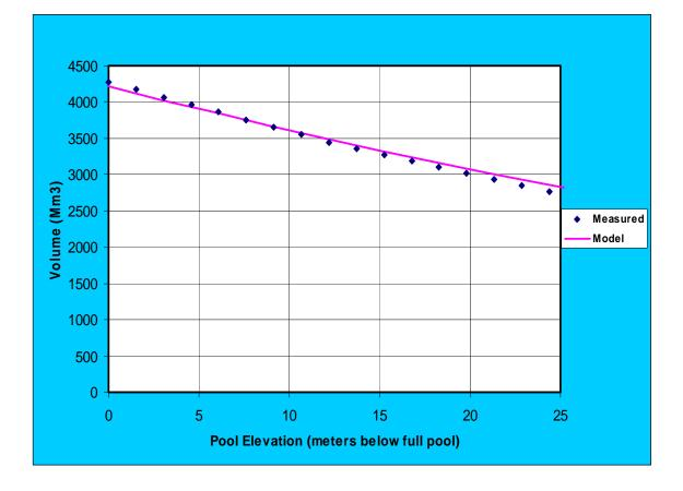
Figure 8. Modeled and observed reservoir volumes for Dworshak Reservoir
