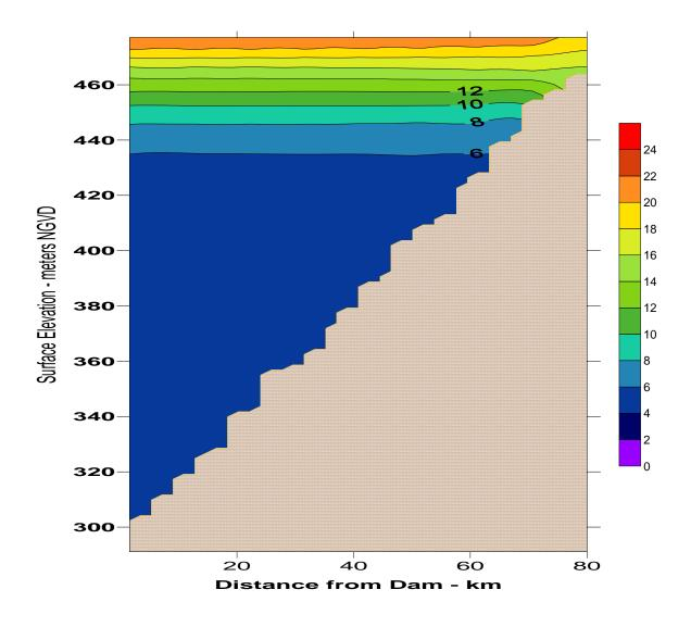
Figure 21. Simulated longitudinal temperature profiles in Dworshak Reservoir on August 8, 2002.
