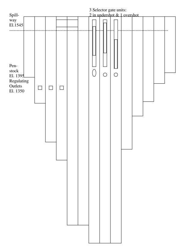
Figure 2. Dworshak Dam face, looking from upstream to downstream
