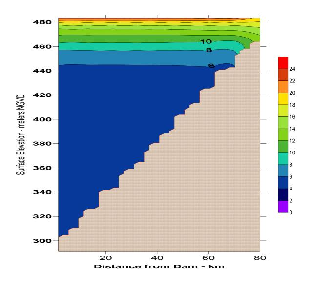
Figure 20. Simulated longitudinal temperature profiles in Dworshak Reservoir on July 20, 2002.
