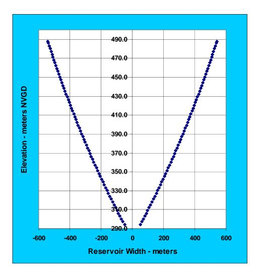
Figure 7. Typical reservoir cross-section based on an exponential shape
