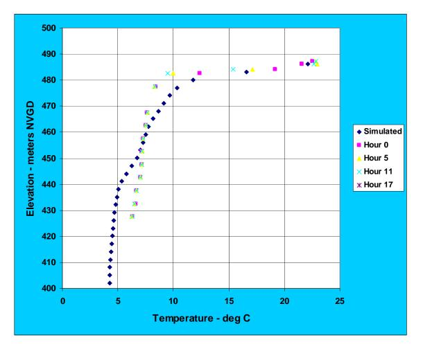
Figure 15. Simulated and observed water temperatures in Dworshak Reservoir at Dworshak Dam on June 30, 2002
