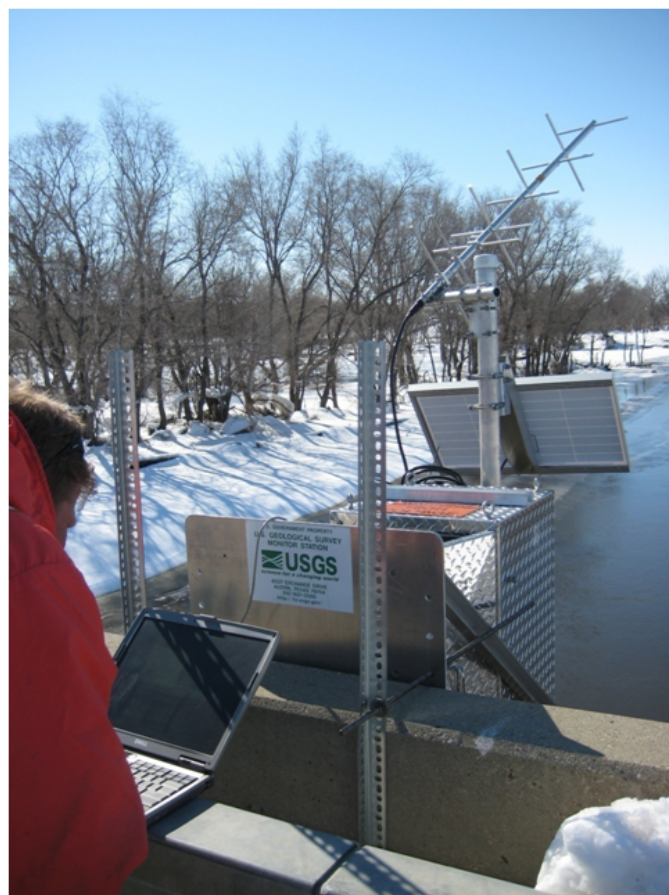
The installation of a rapid deployment gage on the James River near Adrian, North Dakota, during the spring of 2009. Fourteen of these mobile gages were placed on rivers and streams in the James River Basin to help U.S. Army Corps of Engineers track high flow in the basin. A more comprehensive view of developing flood situations can be obtained when these temporary gages are used in conjunction with permanent streamgages in a hydrologic monitoring network. Photograph by Kathleen Rowland, U.S. Geological Survey.
