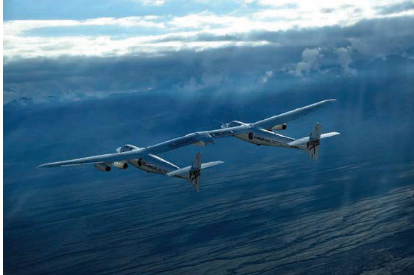
Figure 1: Mothership Carrier Aircraft, VMS EVE
