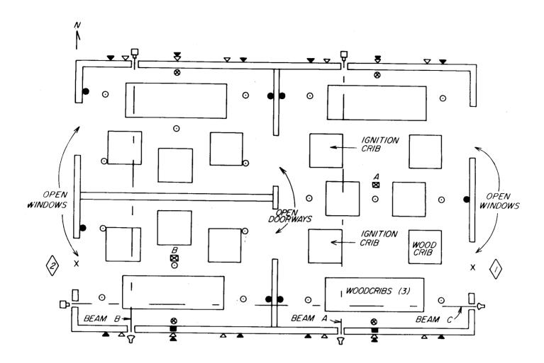
Figure 2.—Plan view of sandwich and wood-frame test structures showing locations of wood cribs, thermocouuples, gas sampling points, and smoke-measuring apparatus.
