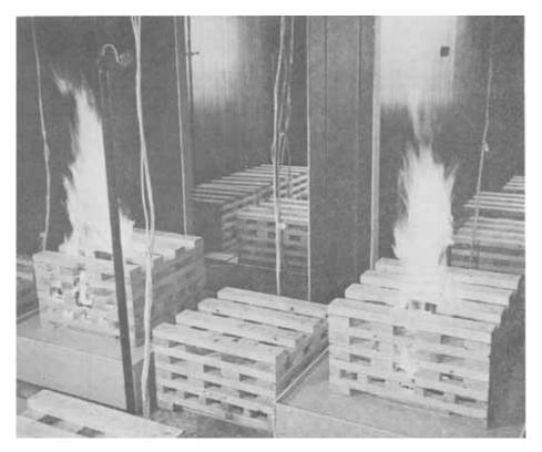
Figure 3.—Ignition cribs shortly after the start of the test—Structure 7. White, beaded wires are thermocouple "frees." Pipes at center of rear room and at the far left are for gas sampling. (M 143767-4)
