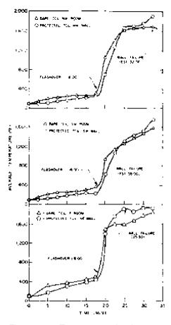
Figure 8. — Temperature development in Structure 7. (M 148 024)
