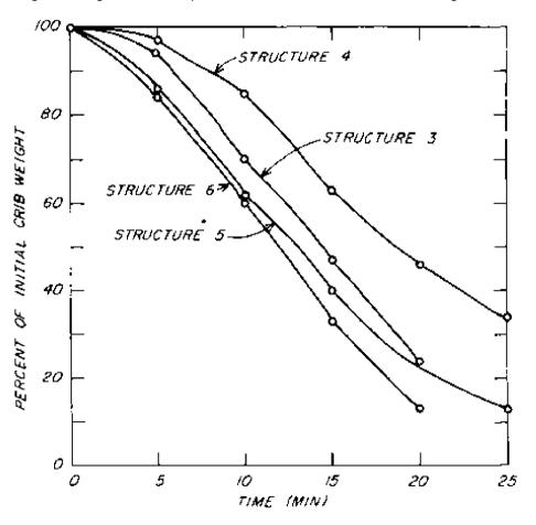
Figure 9.—Percentage of initial crib weight versus time for Structures 3, 4, 5, and 6. Data are the average of the two ignition cribs.
