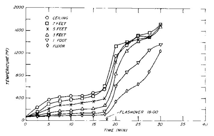
Figure 13.—Temperature at various heights in center of southwest room in Structure 7. (M 148 019)
