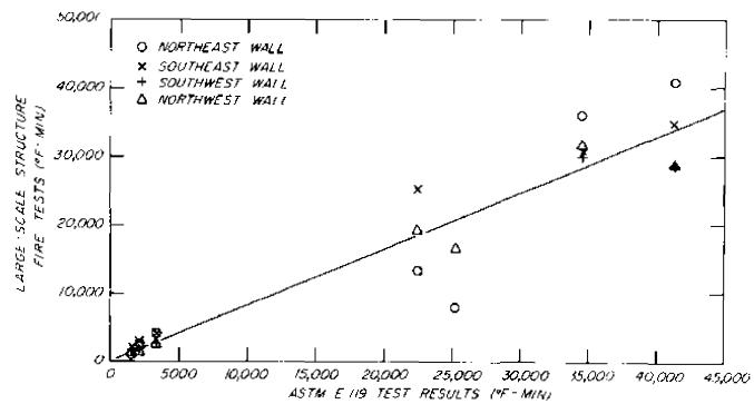
Figure 20.—Areas under the time-temperature curves (average of three protected thermocouples) from ignition to wall failure (see table 11). The two points with ASTM E 119 areas of 25,218° F· minutes are for Structure 2. Because of instrumentation difficulties, temperature data for Structure 2 are limited and erratic, and the accuracy of the areas is not known.
