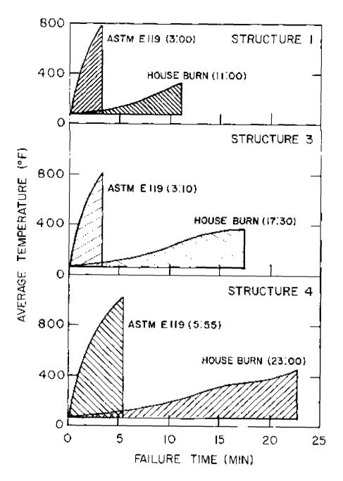
indicate that had-bearing sandwich panels must have thermal protection (e.g., gypsum wallboard) to ensure a reasonable level of fire endurance. It should be noted that the unprotected sandwich panels did give adequate burn-through protection. Thus, unprotected sandwich panels may provide sufficient fire resistance to burn-through in sandwich systems in which the sandwich panel is not a load-bearing component.
