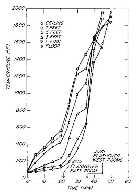
Figure 12.—Temperature at various heights in center of southwest room in Structure 5.
