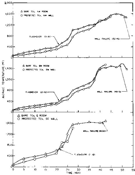
*Figure 7.—Temperaturee development in Structure 5.* (M 148 012)
