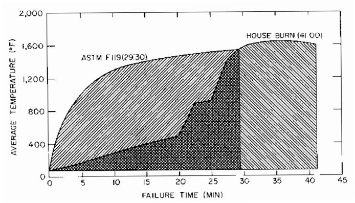
Figure 17.—Time-temperature relationship to time of structural failture for wall construction in ASTM E 119 laboratory test compared to first wall failure (southeast) in full-scale test of Structure 5.
