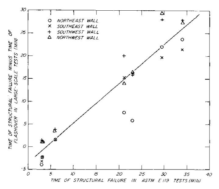
Figure 15.—Time of structural failure minus time of flashover in large-scale tests versus time of structural failure in ASTM E 119 tests (see table 10). (M 148 027)
