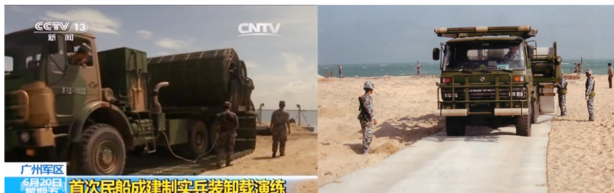
Figure 10. Metal Mat Roadway Installation Shown in the 2014 Exercise Video (left) and Photo from the Harzone Product Catalog of a Fast Soft Road Paver (right) (CCTV/Harzone)
