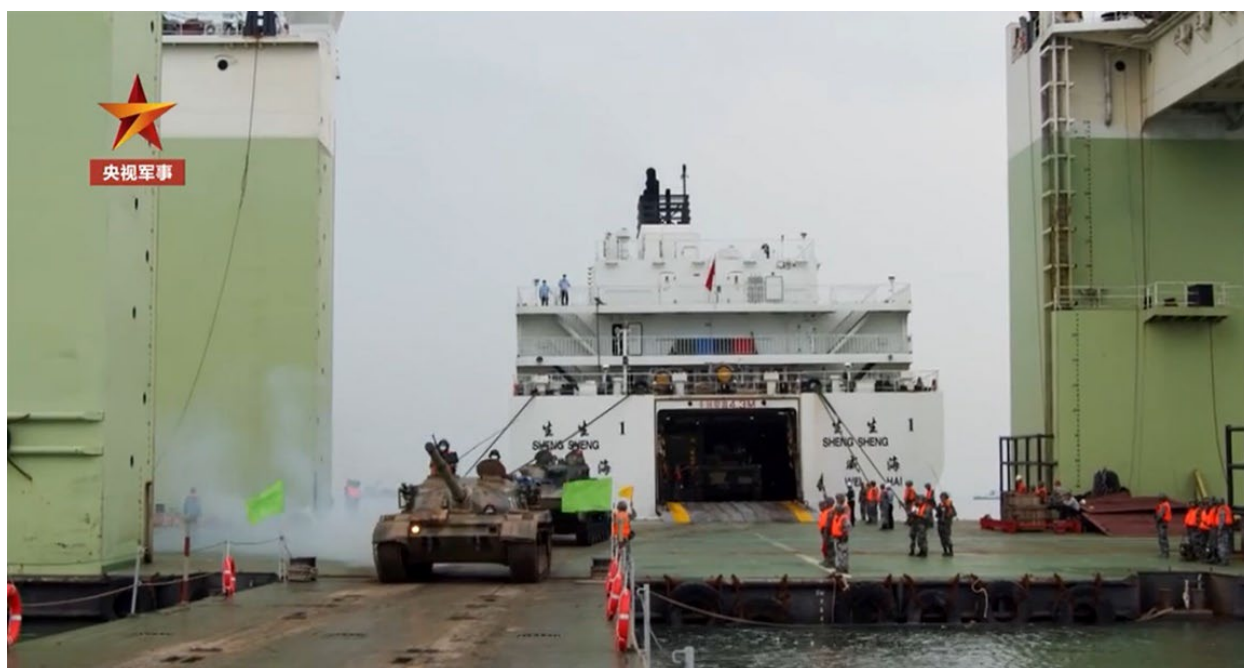
Figure 9. RO-RO Ferry SHENG SHENG 1 Unloading Tanks onto Semi-Submersible Barge and Floating Pier during Exercise EASTERN TRANSPORTATION-PROJECTION 2020A (CCTV)
