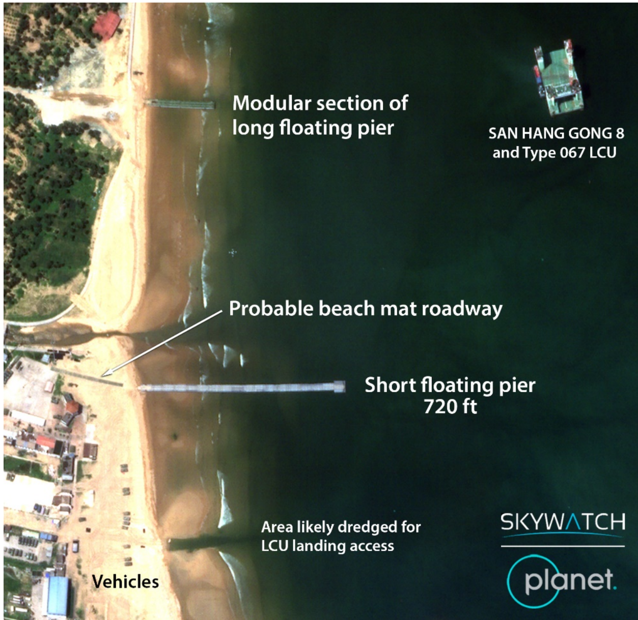
Figure 5. Assembled Short Pier at Lanshan Beach, 11 August 2020 (© 2021 Planet Labs) 25
