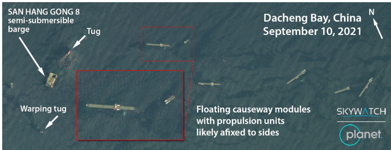
Figure 44. Floating Causeway and SAN HANG GONG 8 Semi-Submersible Barge (© 2021 Planet Labs) 107
