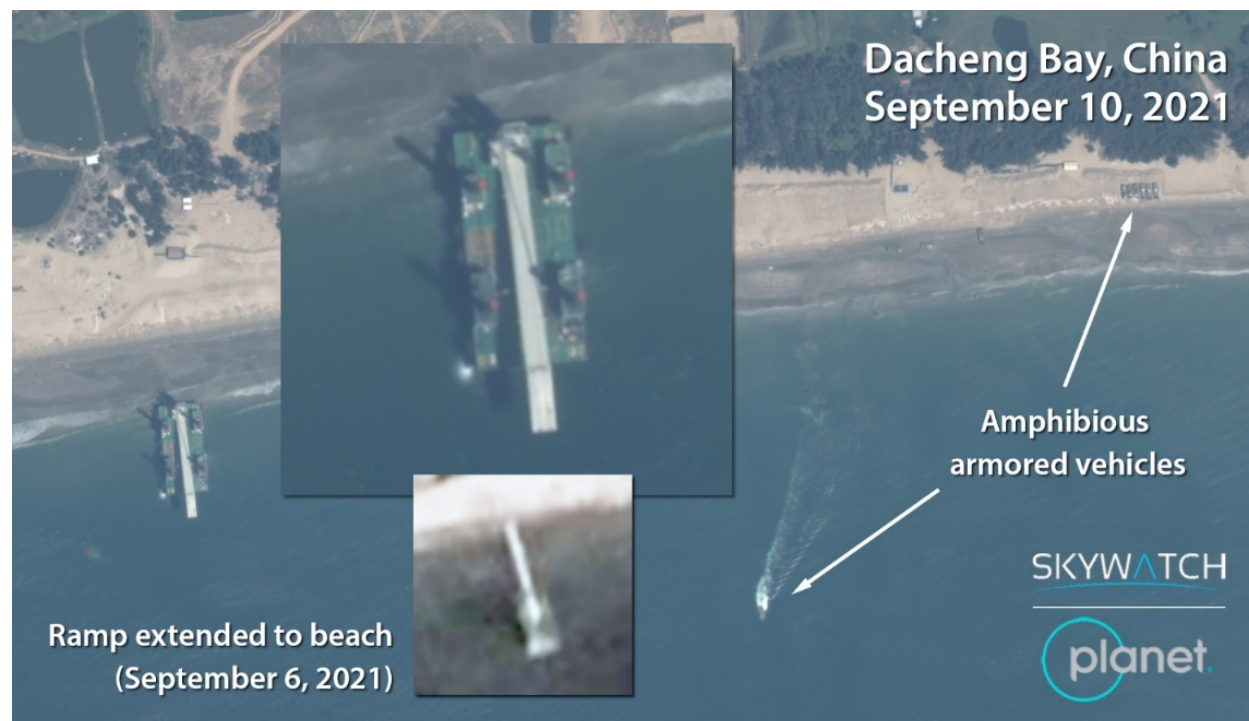
Figure 45. New-Type Landing Platform with 270-foot Extendable Ramp (© 2021 Planet Labs) 109
