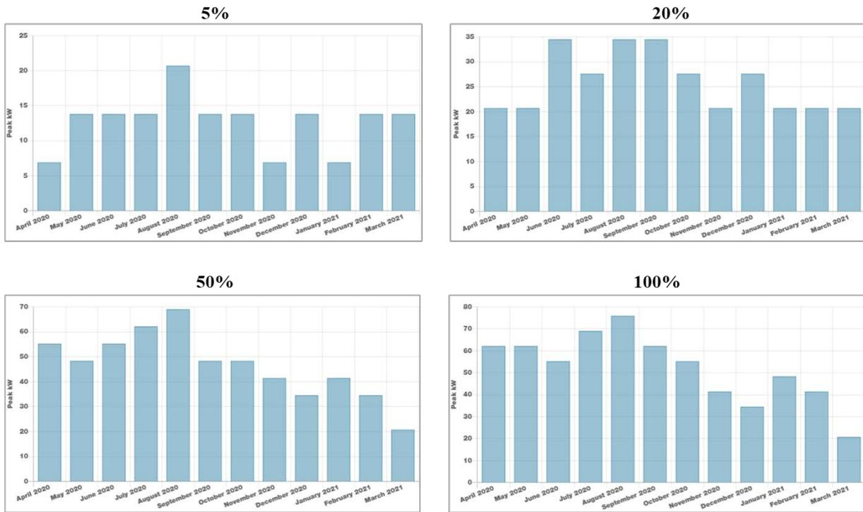
**Figure C-1. Projected monthly peak charging demand at increasing levels of fleet electrification for a single parking facility: UC Riverside**
