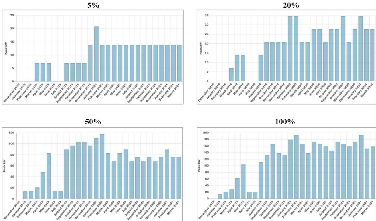
**Figure F-1. Projected monthly peak charging demand at increasing levels of fleet electrification for a single parking facility: UVA**
