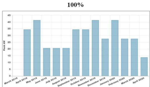
**Figure B-1. Projected monthly peak charging demand at increasing levels of fleet electrification for a single parking facility: UCLA**
