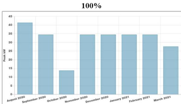
**Figure D-1. Projected monthly peak charging demand at increasing levels of fleet electrification for a single parking facility: CU Boulder**
