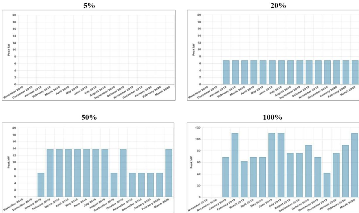
**Figure E-1. Projected monthly peak charging demand at increasing levels of fleet electrification for a single parking facility: UT Knoxville**
