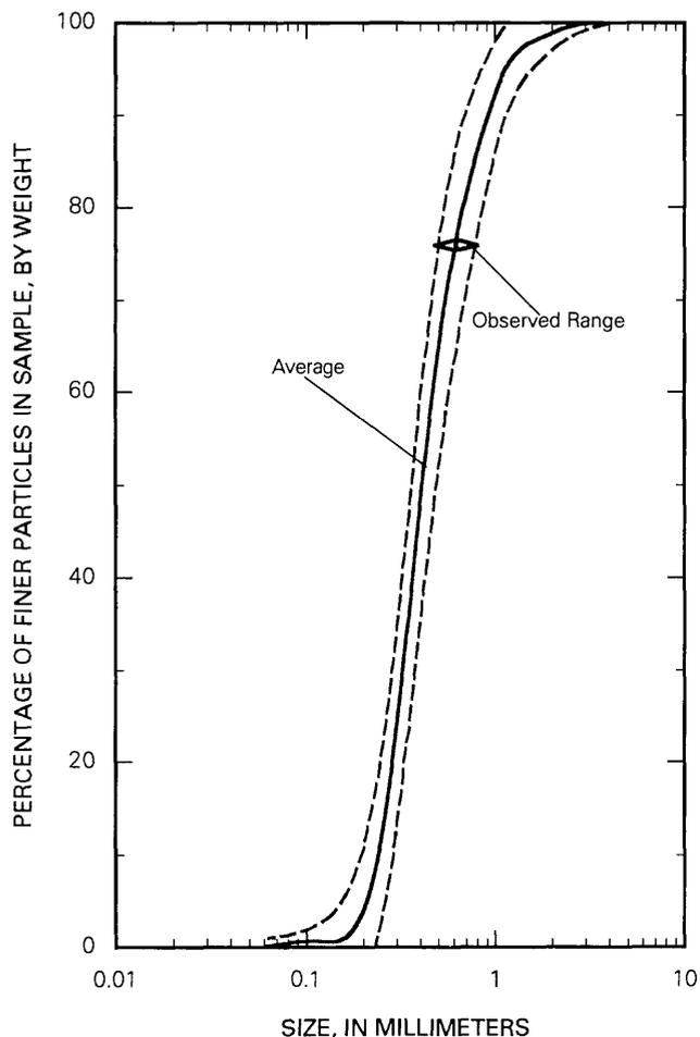
**Figure 11.** Cumulative frequency distribution of average particle size and range of particle sizes in surface bed-material samples from North Fish Creek, site A.
