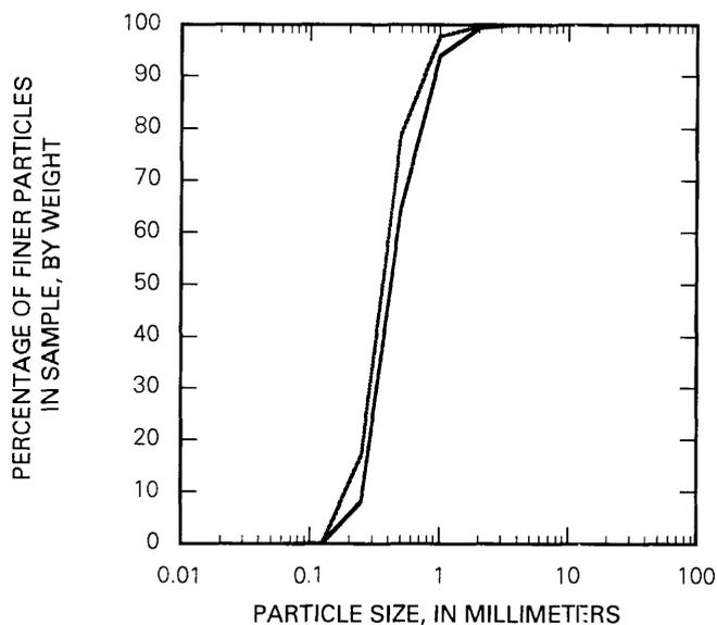
**Figure 12.** Cumulative frequency distribution of particle sizes of two Helley-Smith bedload samples from North Fish Creek, site A.
