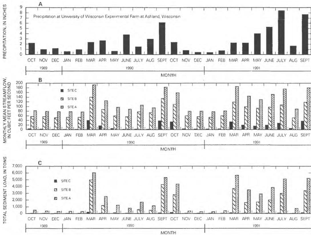
Figure 3. Monthly (A) precipitation, (B) streamflow, and (C) total-sediment load at North Fish Creek, sites A, B, and C, water years 1990-91
