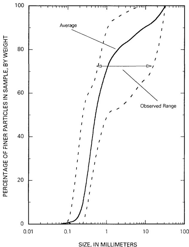
**Figure 7.** Cumulative frequency distribution of average particle size and range of particle sizes in surface bed-material samples from North Fish Creek, site B.
