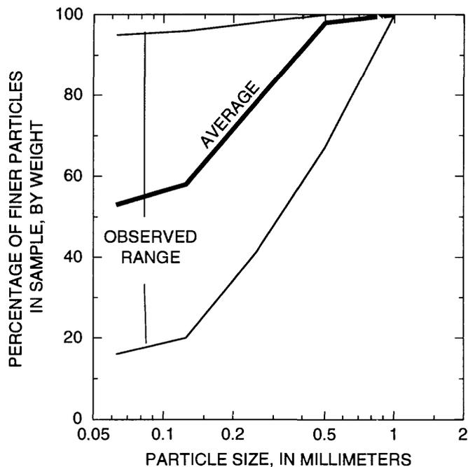
**Figure 10.** Cumulative frequency distribution of average particle size and range of particle size in 20 suspended-sediment samples from North Fish Creek near Ashland, site A, September 1989 through October 1991.
