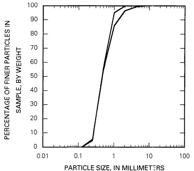
**Figure 8.** Cumulative frequency distribution of particle sizes of two Helley-Smith bedload samples from North Fish Creek, site B.
