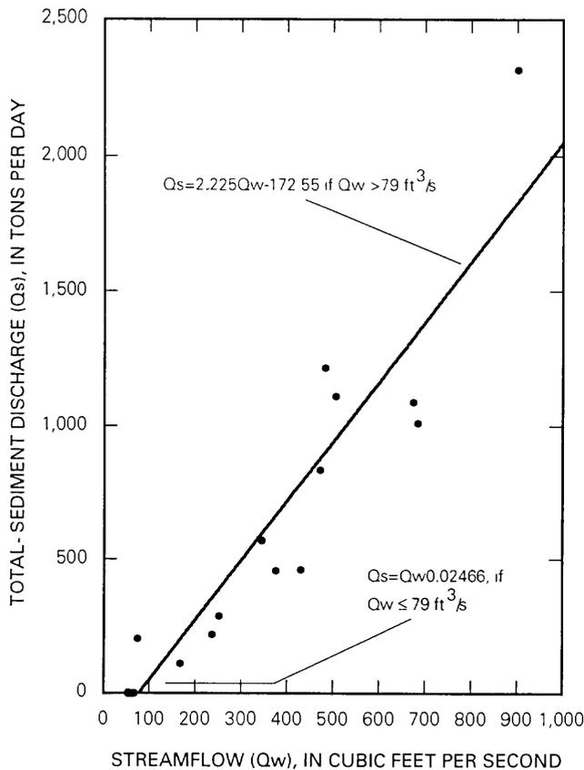
**Figure 5.** Relation of total-sediment discharge to streamflow at North Fish Creek, site B.
