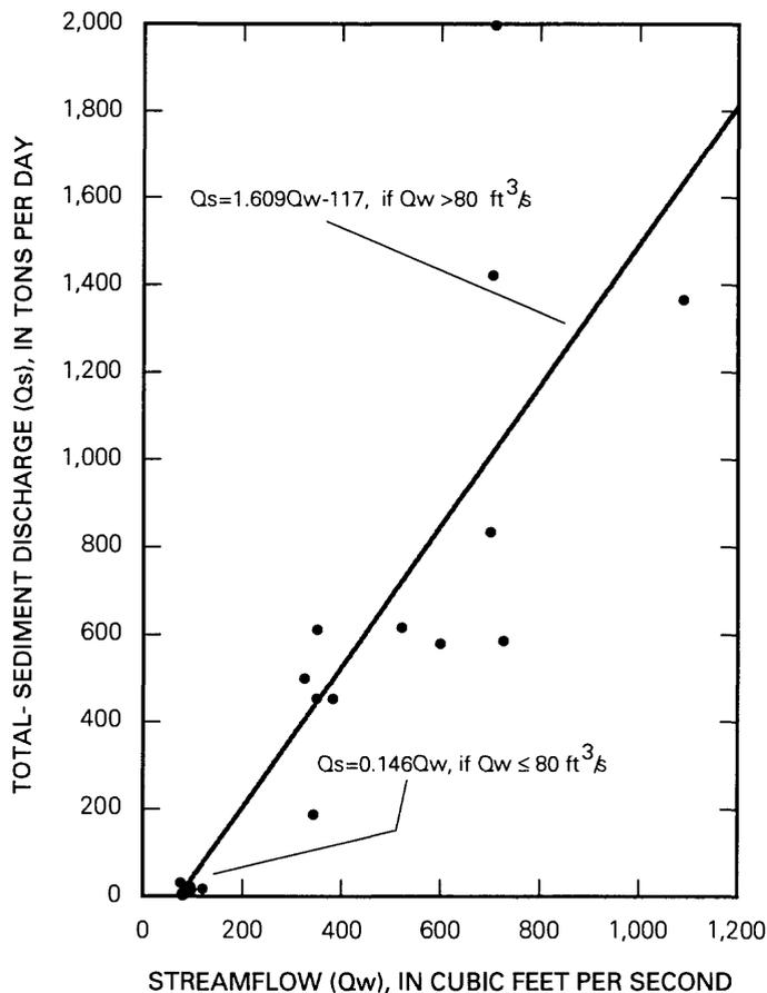
**Figure 9.** Relation of total-sediment discharge to streamflow at North Fish Creek, site A.
