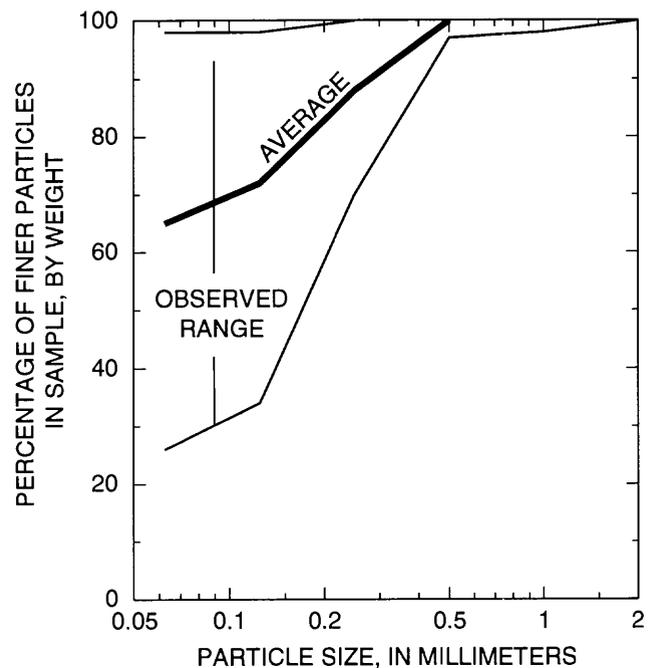
**Figure 6.** Cumulative frequency distribution of average particle size and range of particle size in 20 suspended-sediment samples from North Fish Creek near Moquah, site B, September 1989 through October 1991.
