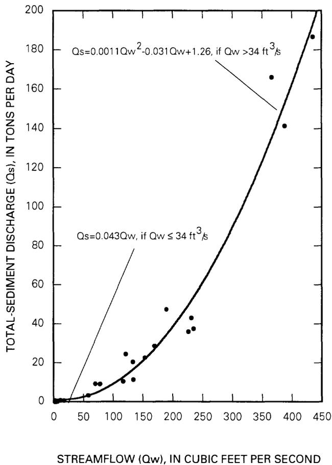
**Figure 4.** Relation of total-sediment discharge to streamflow at North Fish Creek, site C.
