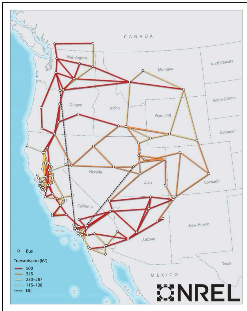
Figure 3. One-line diagram of a simplified WECC 240-bus system
