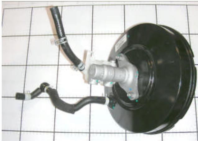
**Figure D-53: Base Brake Booster with Master Cylinder**
