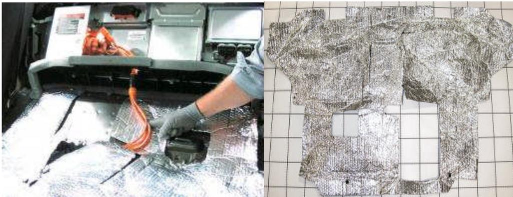
**Figure D-37: Heat Shield for Rear Seat Pan**
