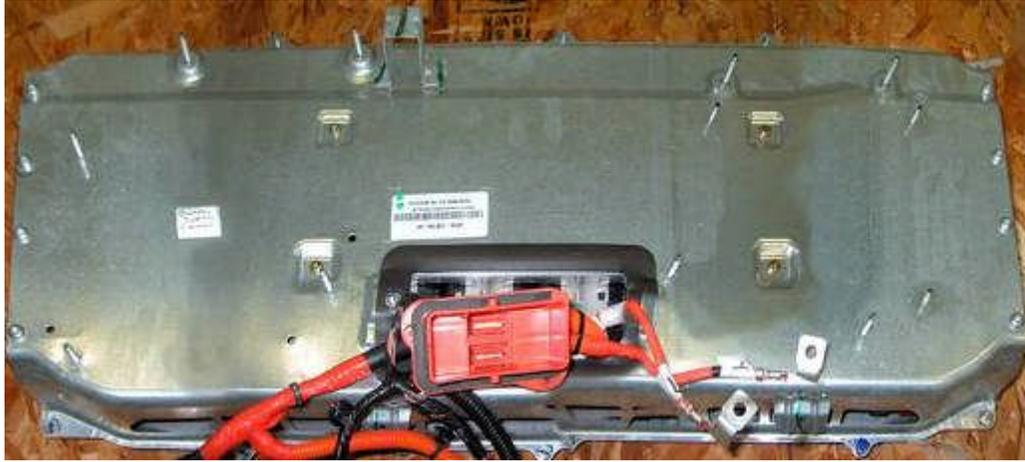
**Figure D-79: Stamped Battery Cover (Cabin side)**
