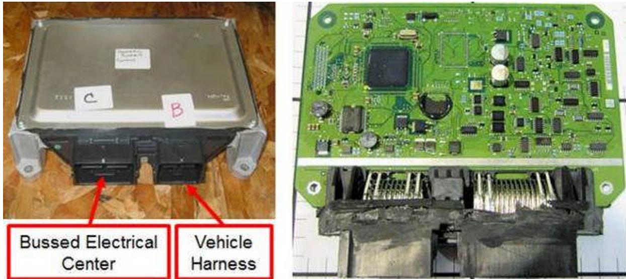
**Figure D-83: The Battery Energy Control Module (BECM)**
