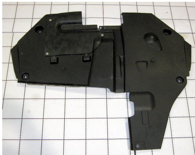
**Figure D-33: Base Fusion, Under Engine Splash Shield**
