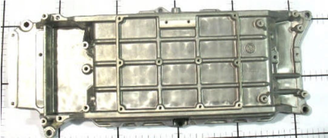
**Figure D-19: Housing, Transmission Control Module**
