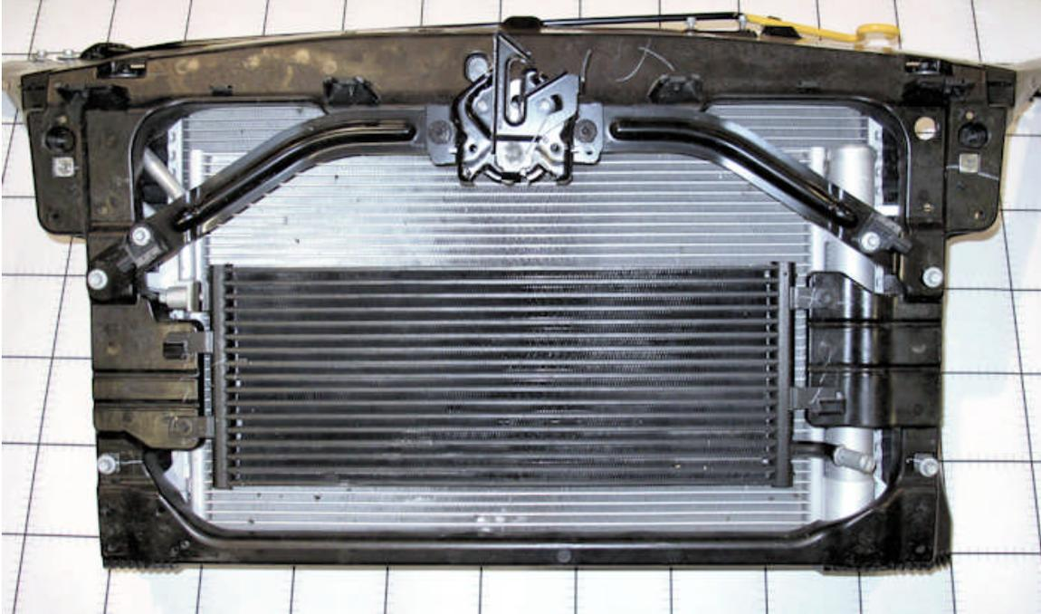
**Figure D-28: Exchanger Mounted to Front End Module (FEM)**
