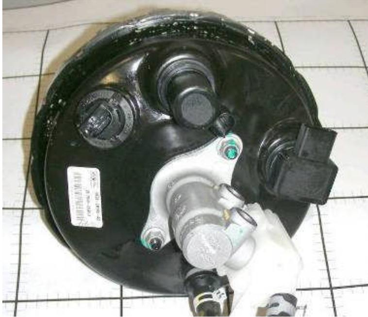
**Figure D-54: Dual Diaphragm Booster**
