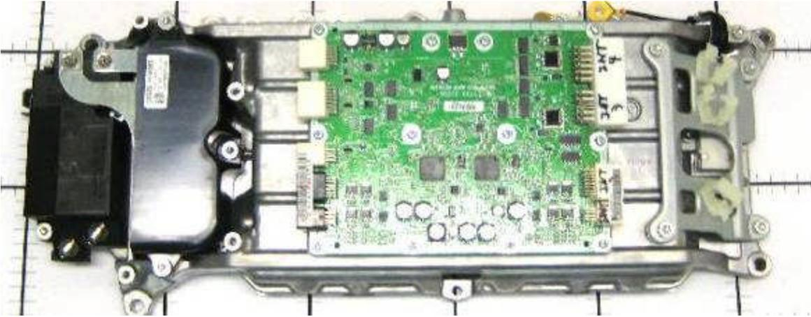
**Figure D-15: Transmission Control Module**
