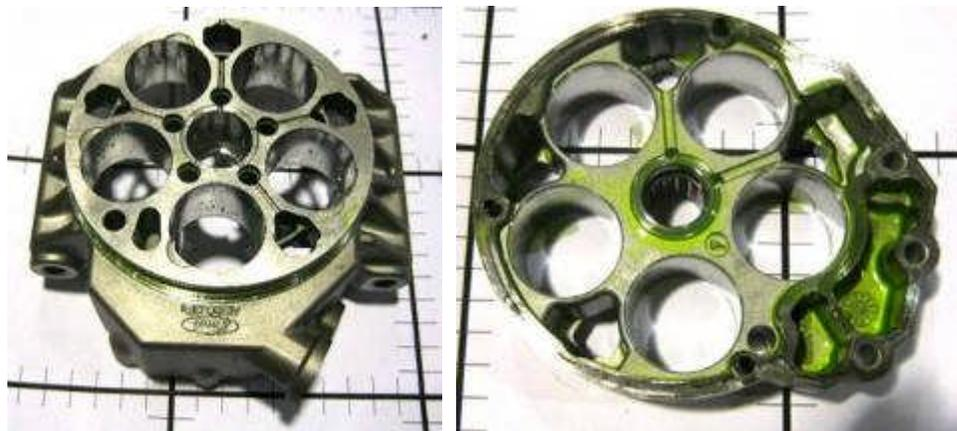
**Figure D-65: AC Compressor Main Housings with Center Bores**
