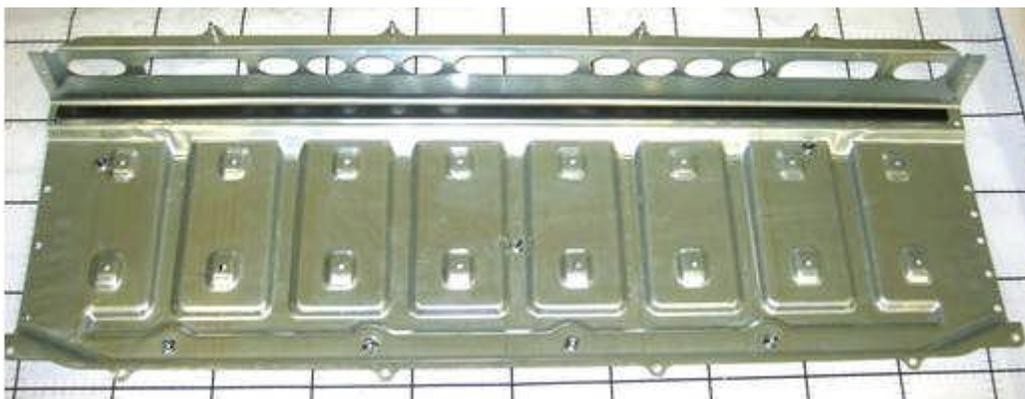
**Figure D-78: Stamped Battery Cover (Under plenum, luggage compartment side)**
