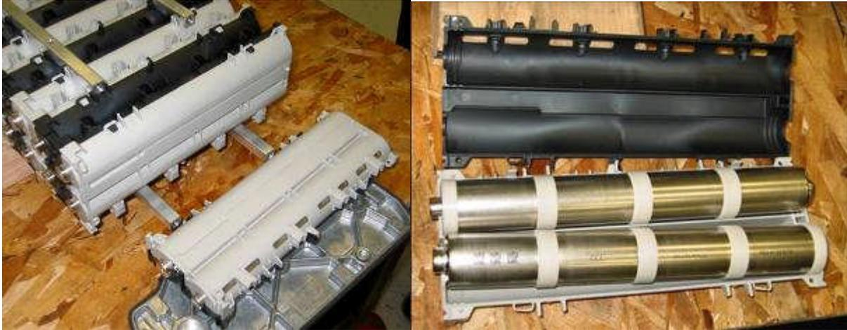
**Figure D-75: NiMH Battery Sub-Modules Contain Eight (8) D-Cells Assemble in Series**
