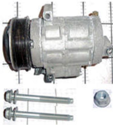
**Figure D-60: Belt-Driven Compressor and Mounting Hardware**
