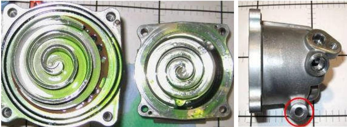
**Figure D-73: Scrolls and Scroll Housing with Mounting Boss for AC Compressor**
