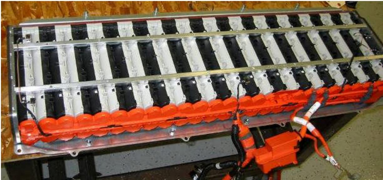
**Figure D-74: NiMH Battery Packs Wired in Series**
