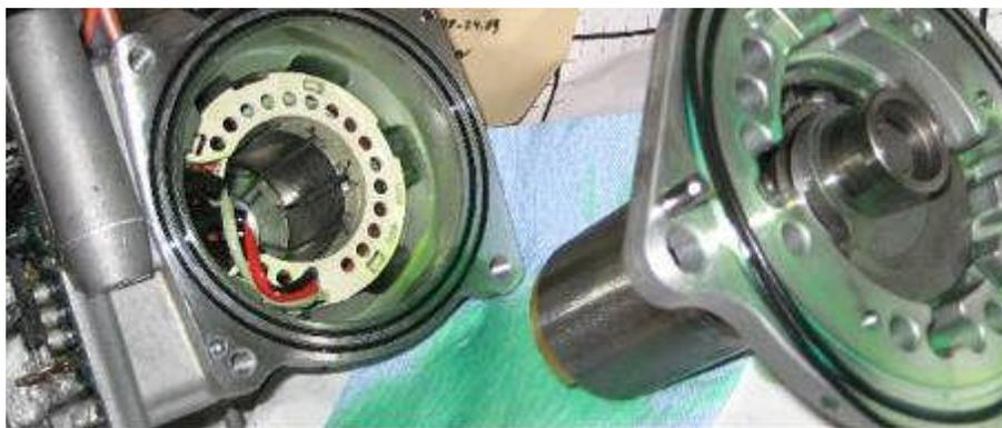
**Figure D-71: Stator and Rotor in Assembly**
