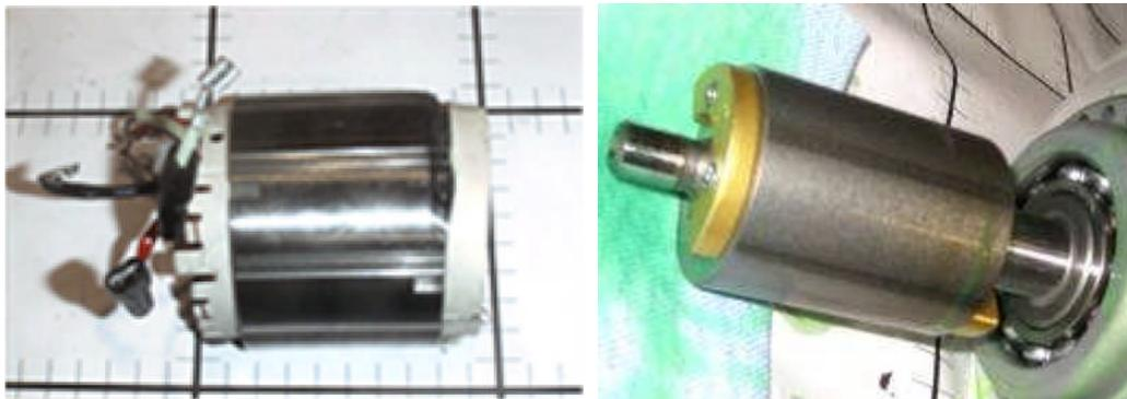
**Figure D-70: Stator and Rotor on Bench**
