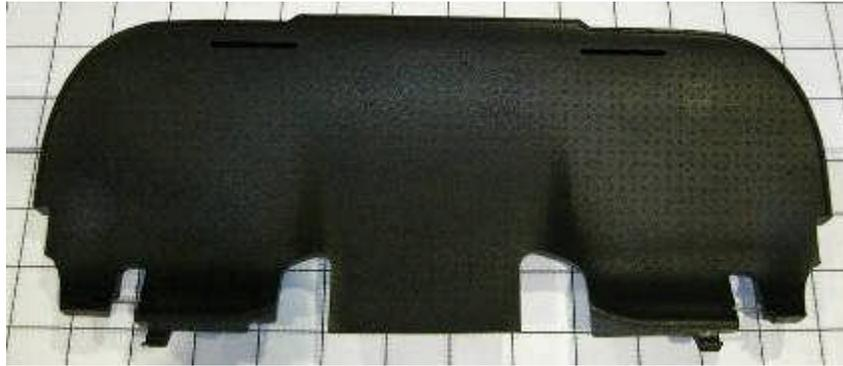
**Figure D-43: Expanded Polypropylene (EPP), Seat Base Structure**
