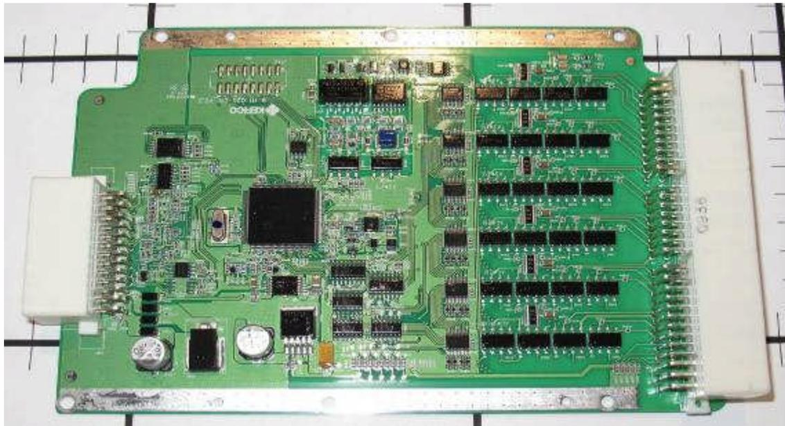
**Figure G-10: The Battery Management Control Board**
