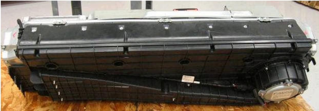
**Figure D-80: Battery Plenum and Cooling Fan (Top rear view)**
