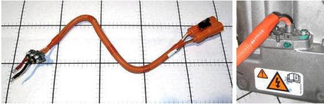
**Figure D-69: High Voltage Low Current (HVLC) AC Compressor Pigtail**
