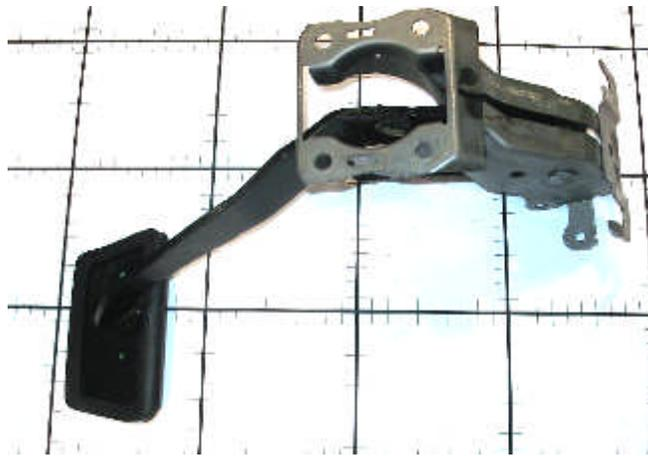
**Figure D-50: Brake Pedal Assembly (Base Fusion)**
