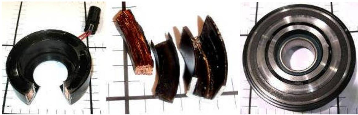
**Figure D-61: Electromagnetic Clutch and Pulley with Bearing**
