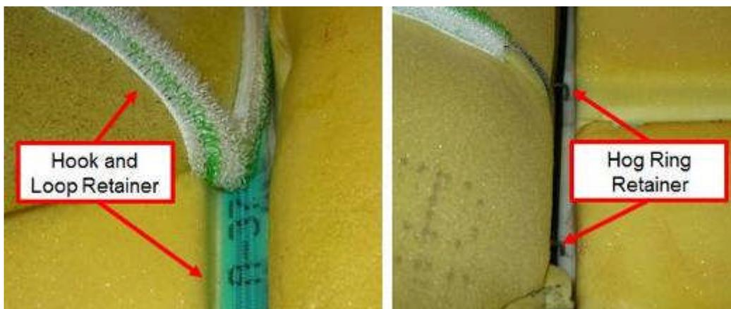
**Figure D-40: Seat Cover Fastening Types**
