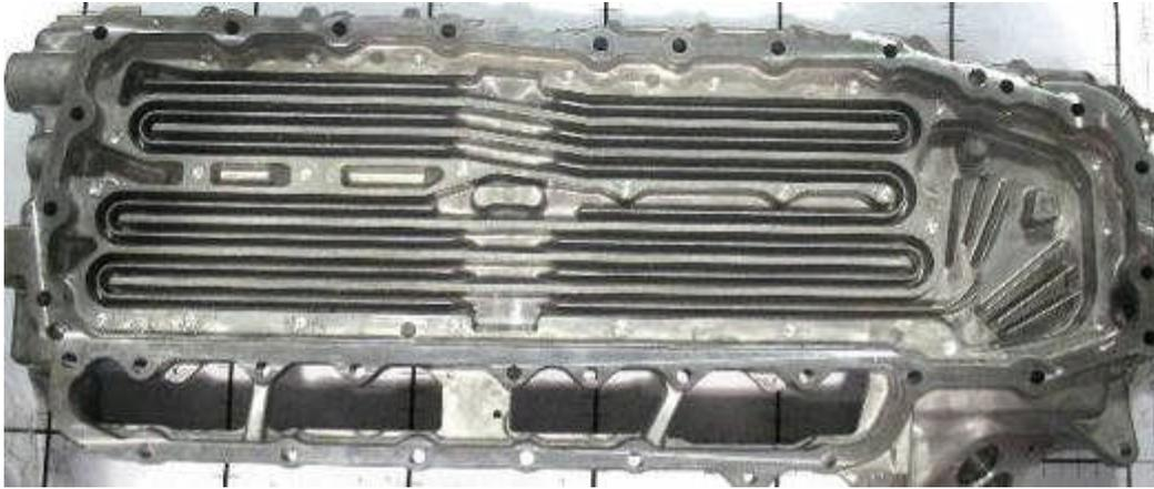
**Figure D-31: Internal Heat Exchanger, Integrated into the Bottom Side of the Housing – Electronic Assembly**
