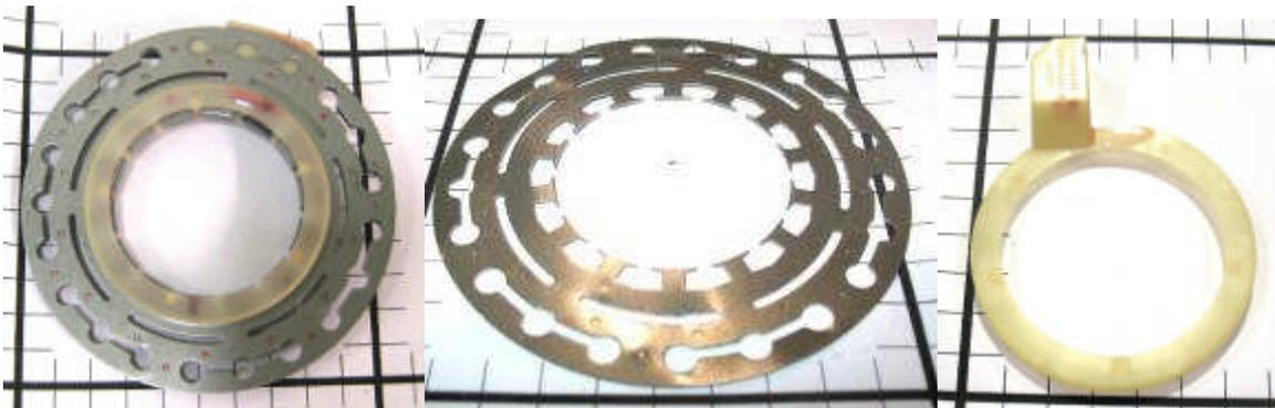
**Figure D-21: Speed Sensor, Generator**
