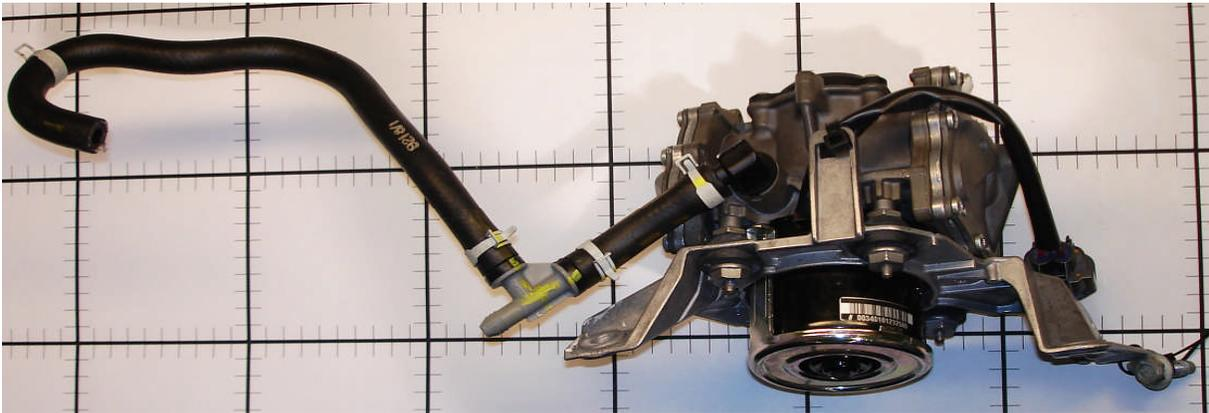
**Figure D-58: Vacuum Pump Assembly**
