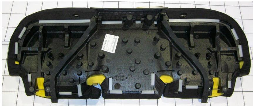
**Figure D-42: Rear Seat Bottom (HEV)**
