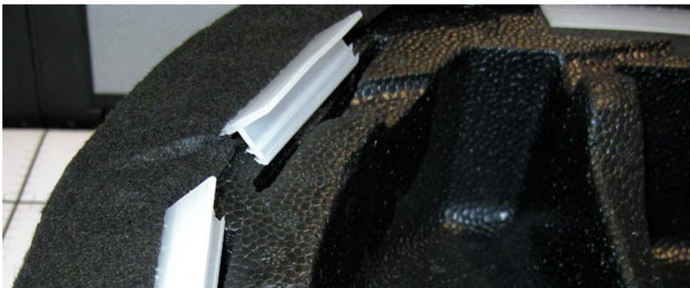
**Figure D-45: Extruded Retainers for Seat Cover to Base**
