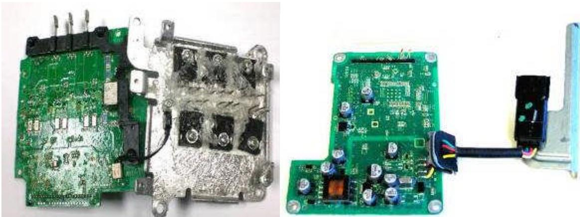
**Figure D-68: Printed Circuit Boards (PCBs) and IGBT Heatsink Plate**
