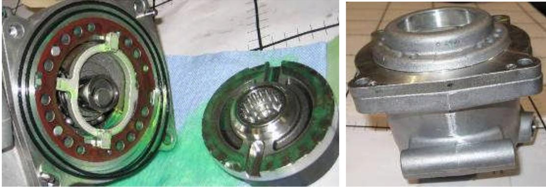
**Figure D-72: Eccentric Drive and Scroll Housing**
