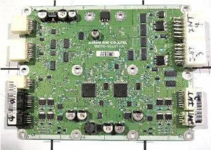
**Figure D-18: CVT Control Circuit Board**
