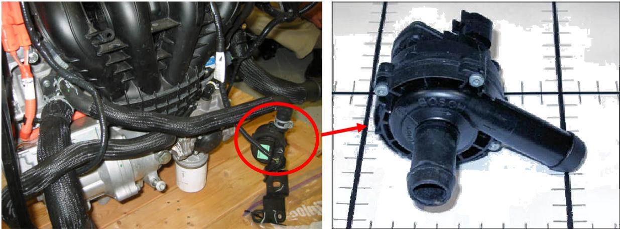
**Figure D-59: Auxiliary Water Pump**
