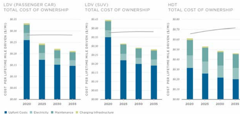
Figure 1: TCO for EVs (bars) vs. ICE vehicles (lines), showing TCO parity achieved by 2023 for LDVs (left and center) and an existing TCO advantage for HDTs (right). Upfront costs include taxes. Maintenance costs of EVs include battery replacement cost.
