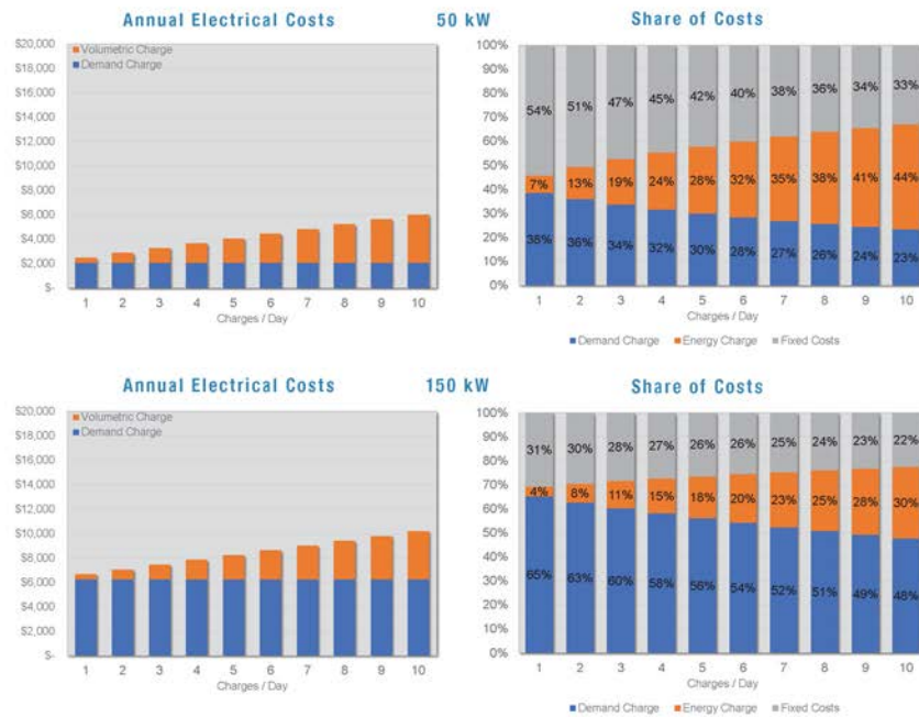
Figure 7. DCFC station costs by charges per day: 50 kW and 150 kW chargers
