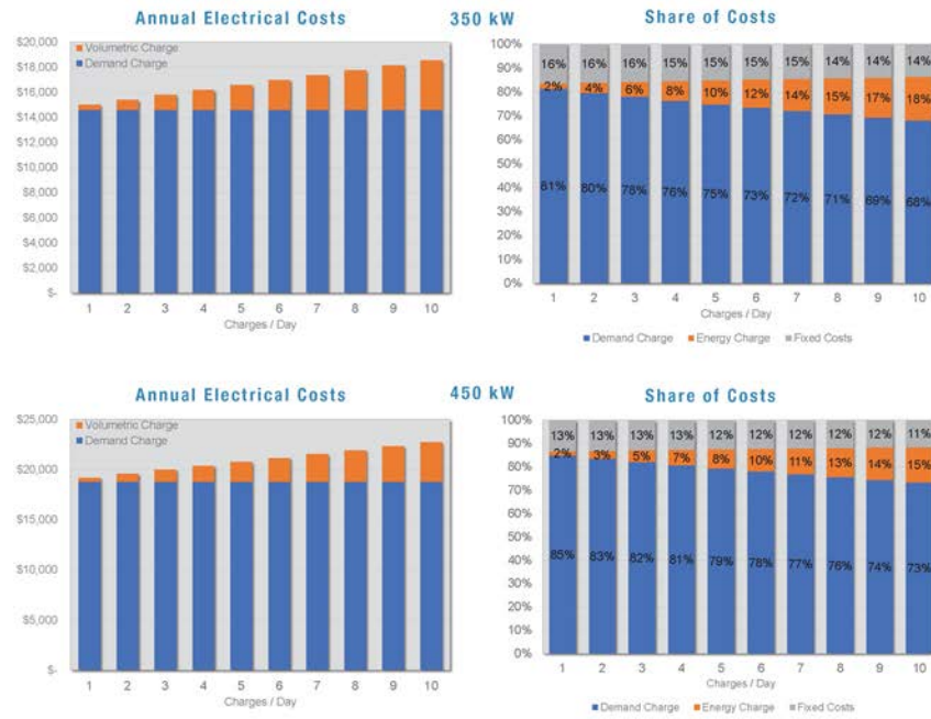
Figure 8. DCFC Station costs by charges per day: 350 kW and 450 kW chargers
