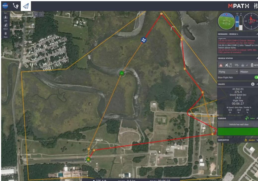
Figure 102: Map view of Flight Track vs. Geofence during Test Run 3 on March 30<sup>th</sup>
