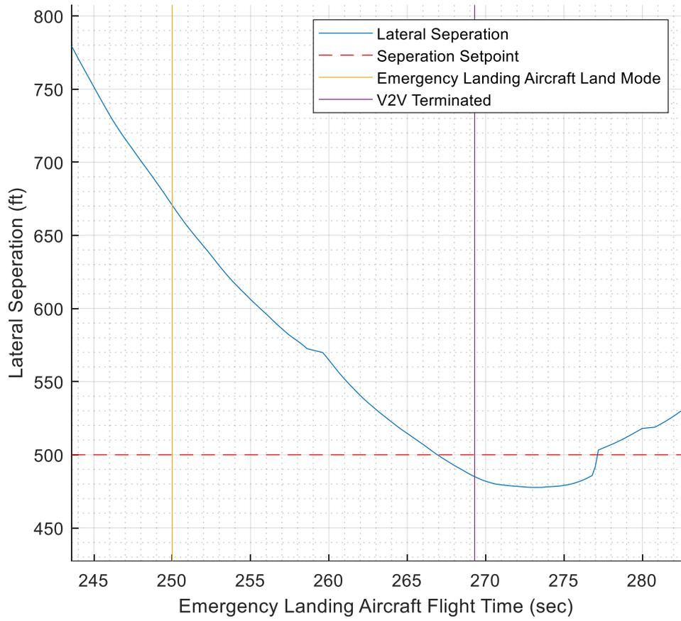
Figure 52: Lateral Separation Plot of Test Run 3 ATAM on April 26<sup>th</sup>
