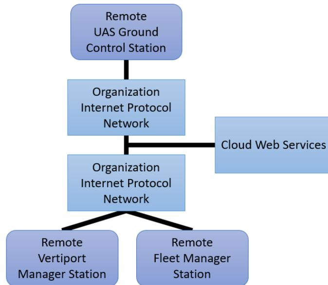
Figure 11: High Level Traffic Management Data System Diagram
