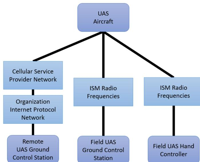
Figure 10: High Level C2 System Diagram
