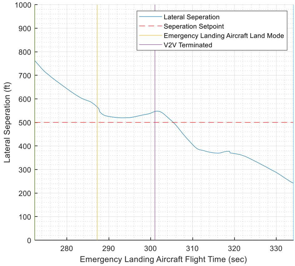
Figure 75: Lateral Separation Plot on Test Run 2 ATAM on April 21<sup>st</sup>
