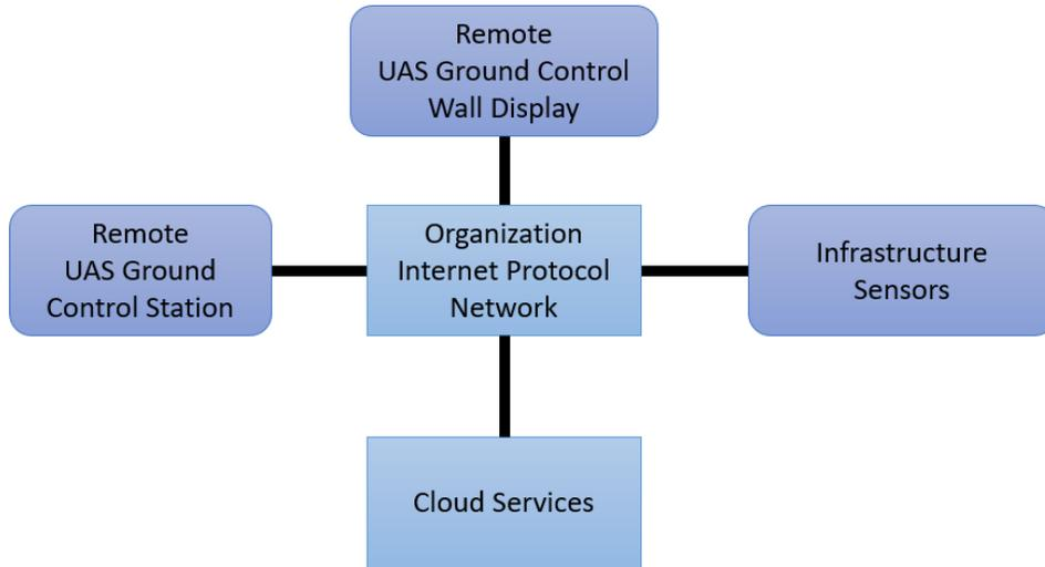
Figure 12: High Level Remote Operator Data System Diagram
