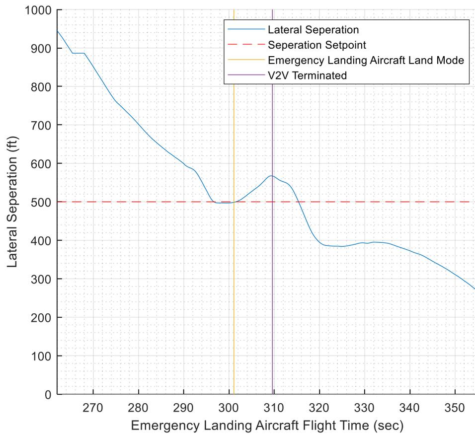
Figure 84: Lateral Separation Plot on Test Run 4 ATAM on April 26th 2022
