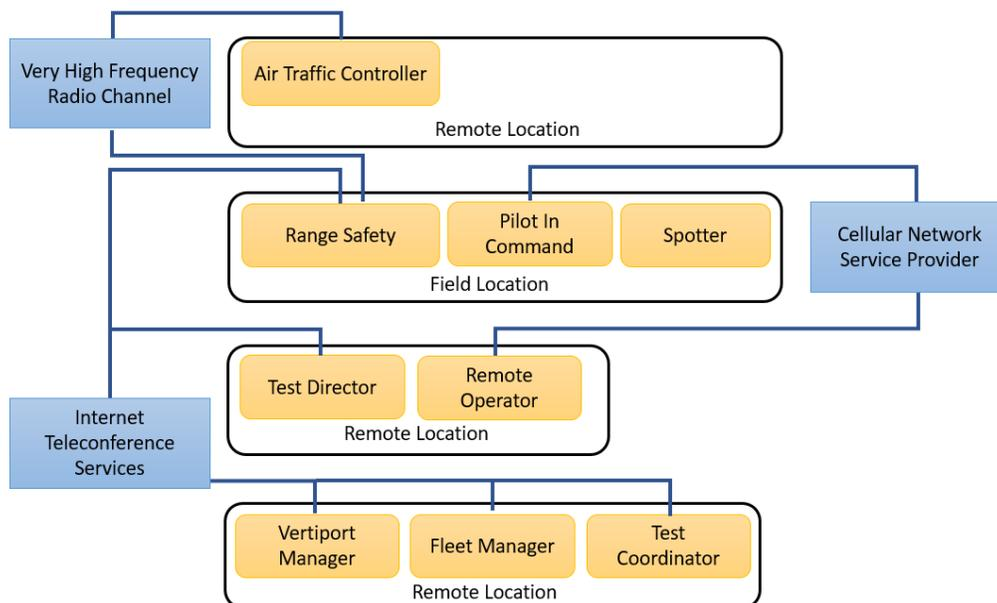
Figure 13: Voice Communications System Diagram
