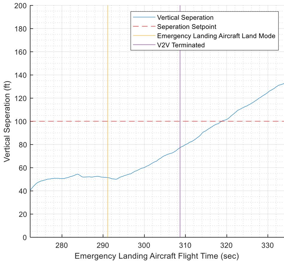
Figure 65: Vertical Separation Plot of Test Run 2 ATAM on April 5<sup>th</sup>
