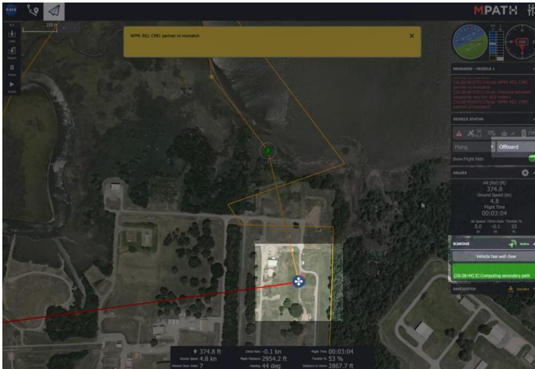
Figure 100: Geofence Avoidance Maneuver Display on GCS
