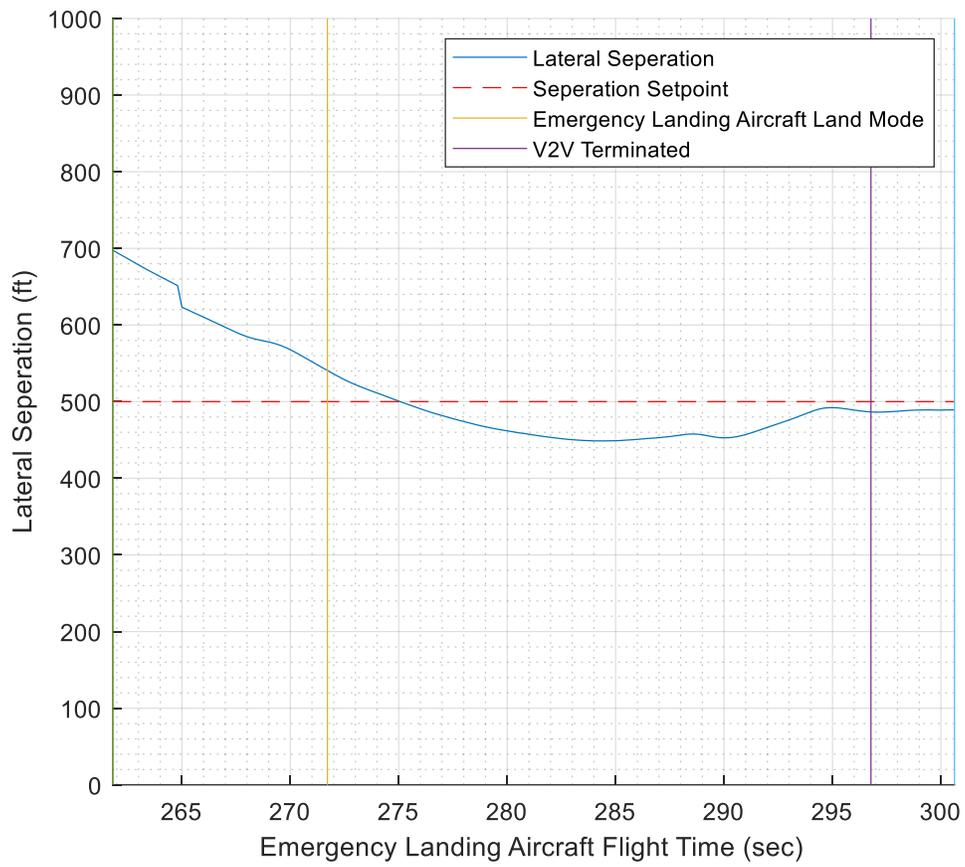
Figure 34: Lateral Separation Plot during Test Run 3 ATAM on April 12<sup>th</sup>
