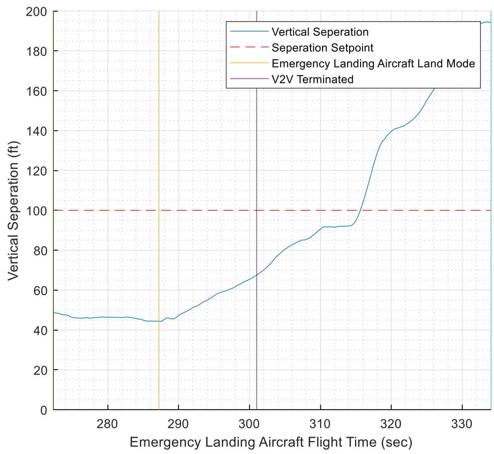
Figure 74: Vertical Separation Plot for Test Run 2 ATAM on April 21<sup>st</sup>
