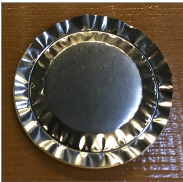
Figure 11. Pd/Ag membrane removed from sensor after exposure to HTF vapor at 400°C.
