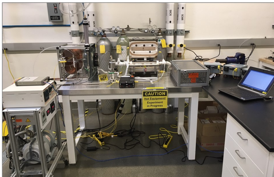
Figure 45. Laboratory test layout for testing the integrated hydrogen sensor and separation module.
