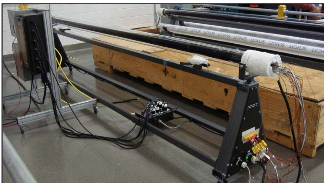
Figure 16. NREL heat-loss test stand for daily heating of in-service receiver.
