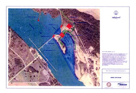
The Lock and Dam #14 facility currently consists of an earthfill embankment, a navigation lock (with a normal lift of 20 feet), and a gated spillway. The spillway is formed by a low concrete apron about 840 feet long, surmounted by twelve 60-foot by 21-foot Tainter gates.
