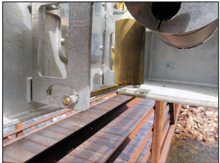
Figure 19. Wire-weight gages mounted on bridges.
