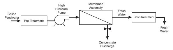
Figure 1. Schematic diagram of a BWRO unit.
