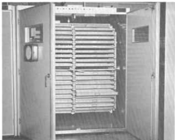
Figure 11.—Modern incubator. Drum is reversed automatically every 3 hours to turn eggs. Humidity indicator and temperature recording device are in door at left.
