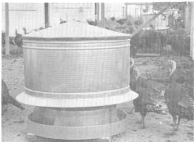
Figure 23. —Large-capacity, portable, hopper-type feeder with rain guard for turkeys over 8 weeks old. (Photo from Colorado State University.)
