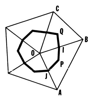
Figure 5. Control volume using cell bisectors.
