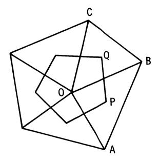
Figure 4. Alternative control volume for Jameson's scheme.
