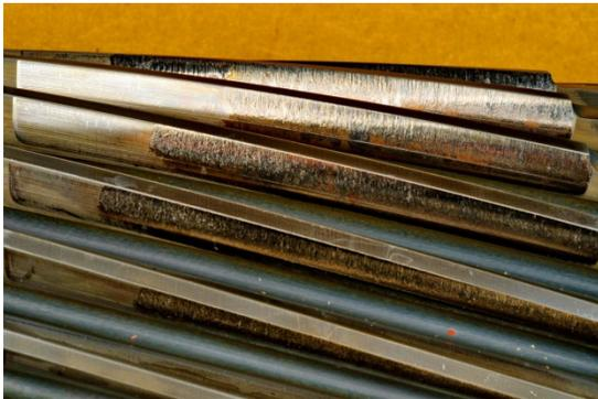
Figure 7: Pinion damage on the 750-kW gearbox HSS. Photo from GEARTECH, NREL / 19743.
