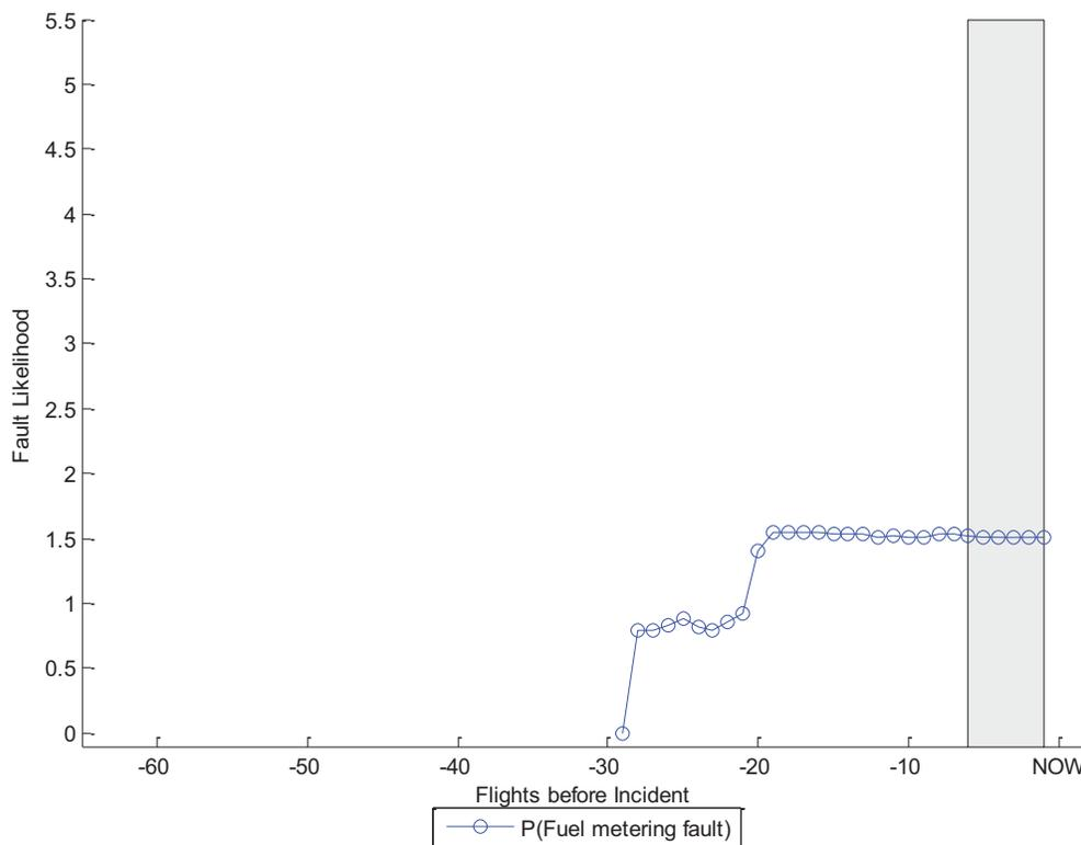
**Figure 23: Fault prediction using the Rising Start trend monitor**
