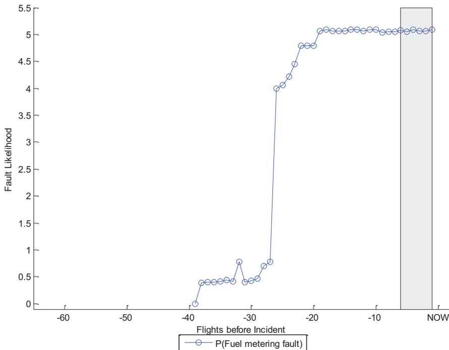
**Figure 27: Fault prediction fusing all three monitors**
