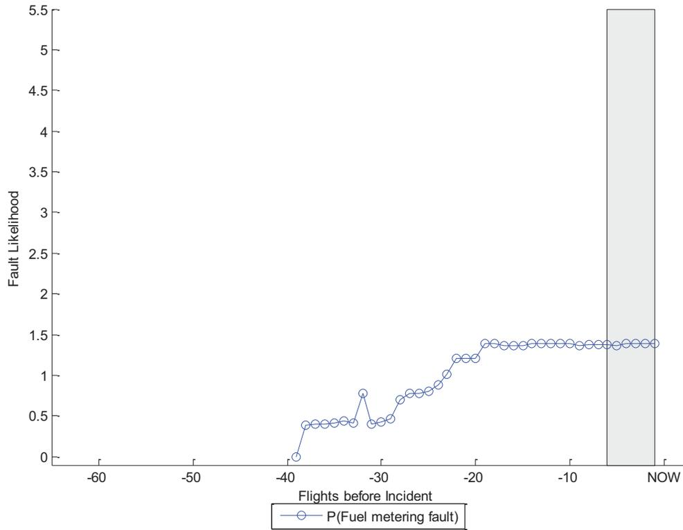
**Figure 25: Fault prediction from fusing results from the Rising Start and Fast Start trend monitors**
