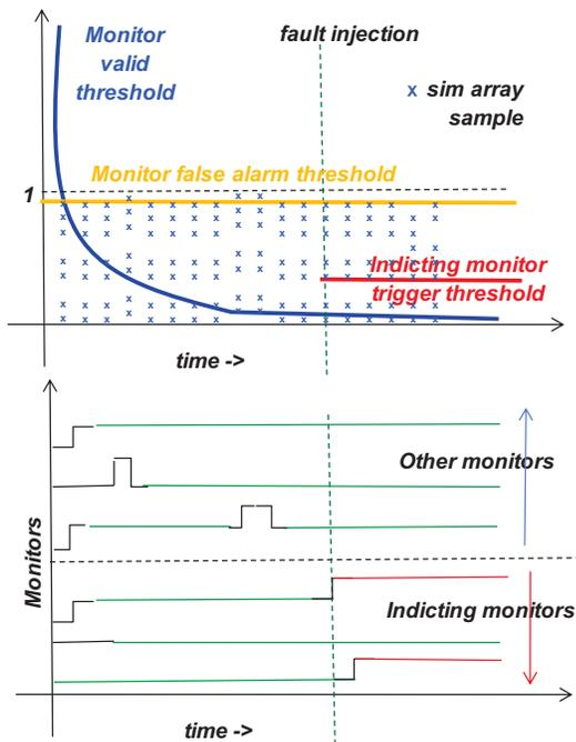
Figure 9: (a) Three thresholds for monitor generation; (b) Diagnostics monitors
