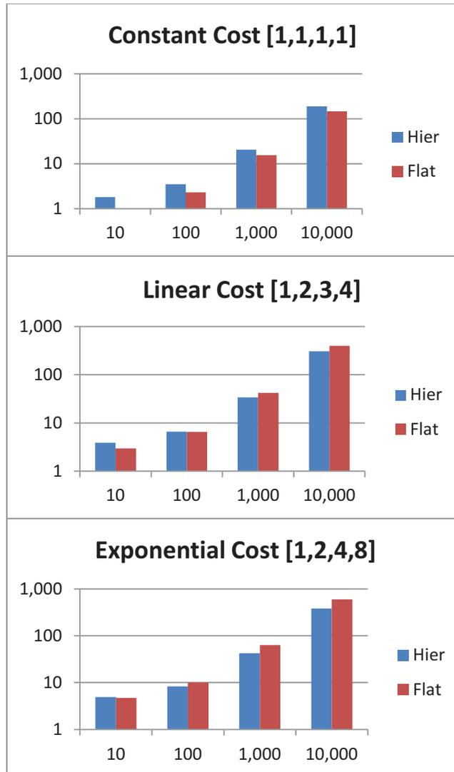
Figure 21: Relative cost of hierarchical and flat reference models
