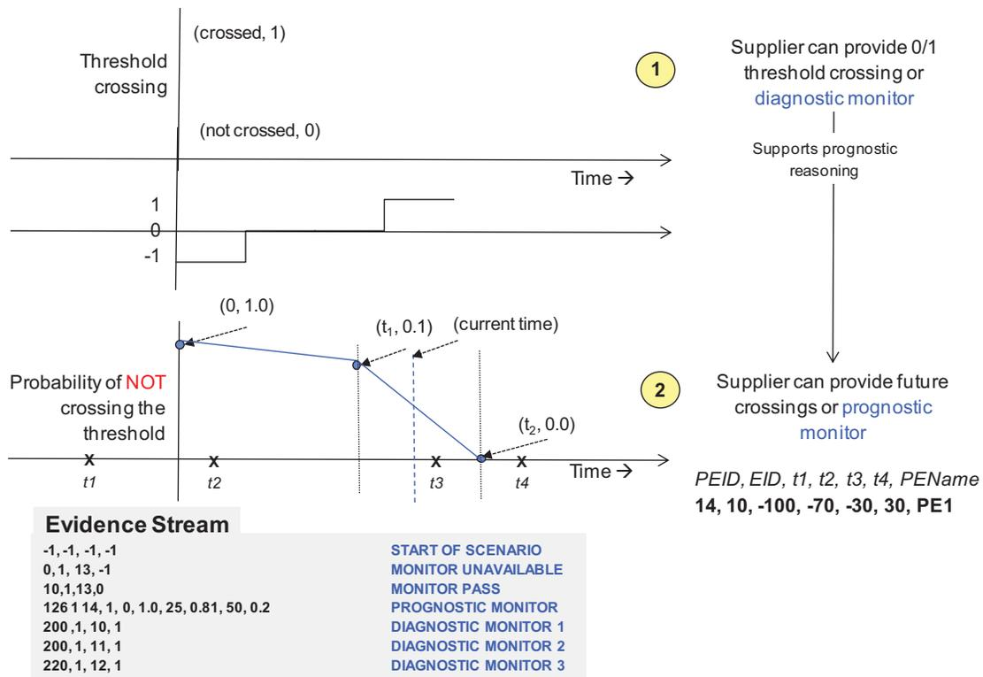
Figure 10: Types of evidence generated by the failure mode simulator
