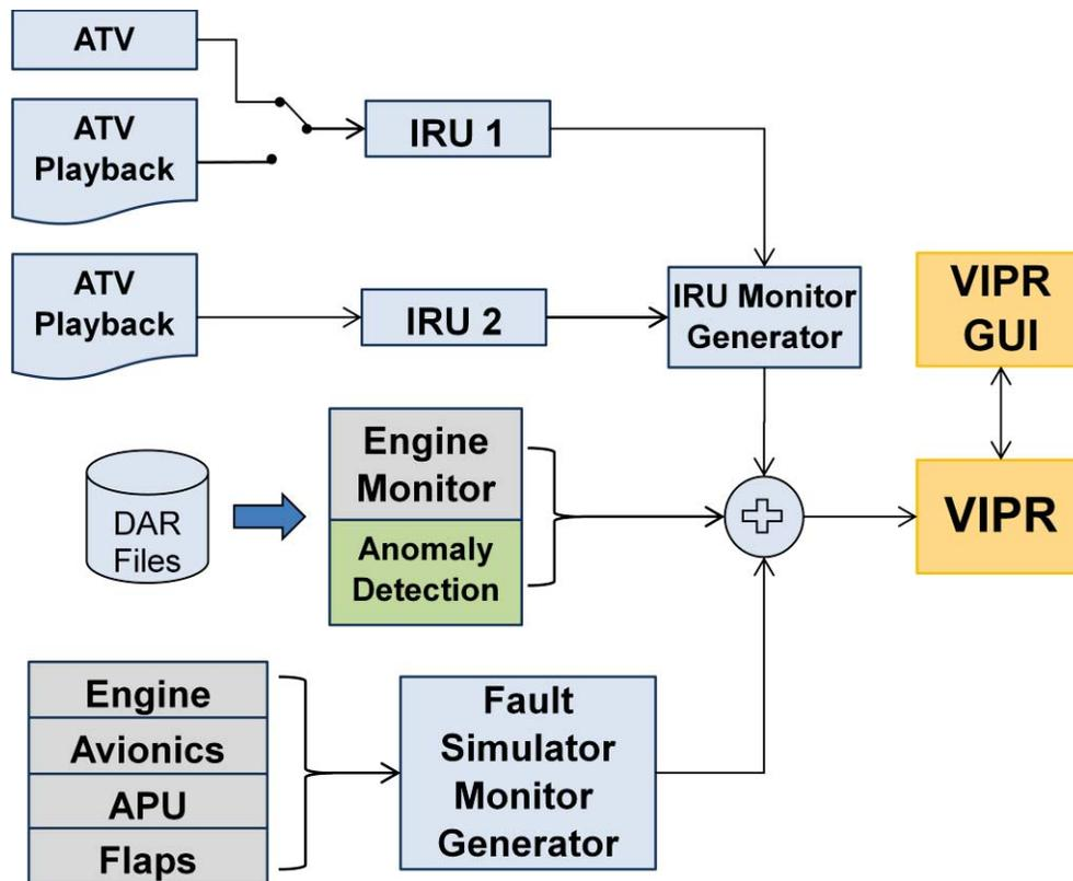
Figure 28: The logical architecture of the VPR Hardware-in-the-Loop demonstration.
