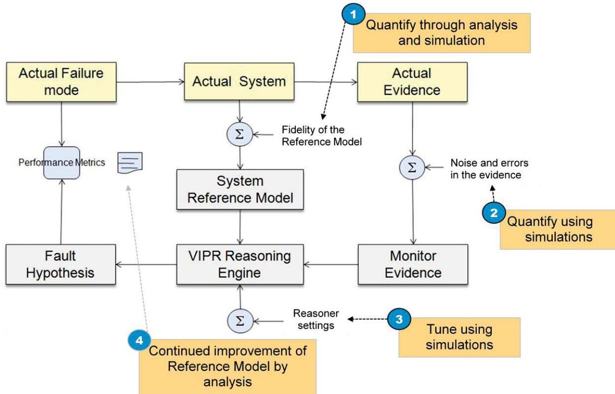
**Figure 6: VIPR Data Flow Showing Four Opportunities for Evaluating Results and Refining Inputs**
