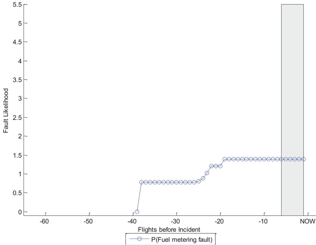
**Figure 24: Fault prediction using the Fast Start trend monitor**
