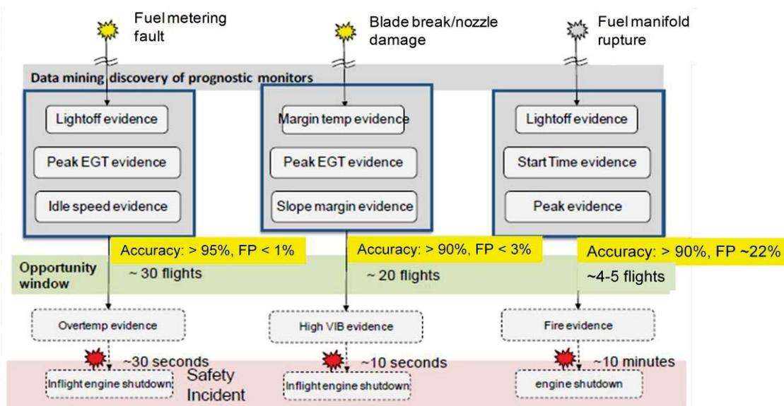
Figure 16: Discovery of prognostic monitors using data mining on an airlines database
