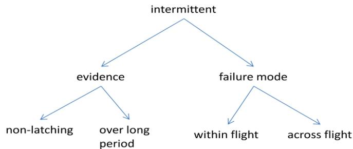
**Figure 4: Types of intermittent faults**
