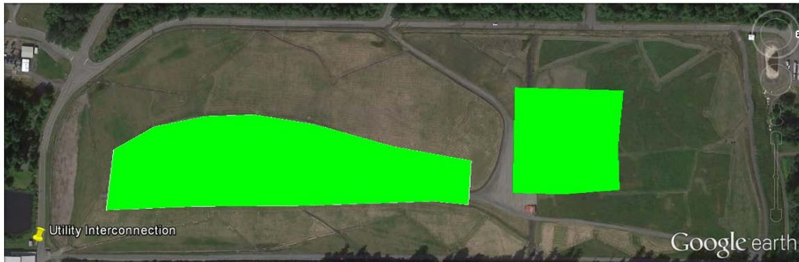
**Figure 6. Aerial view of the feasible area (green) for PV at the Snohomish County Cathcart Landfill site (south is to the left in this image)**
