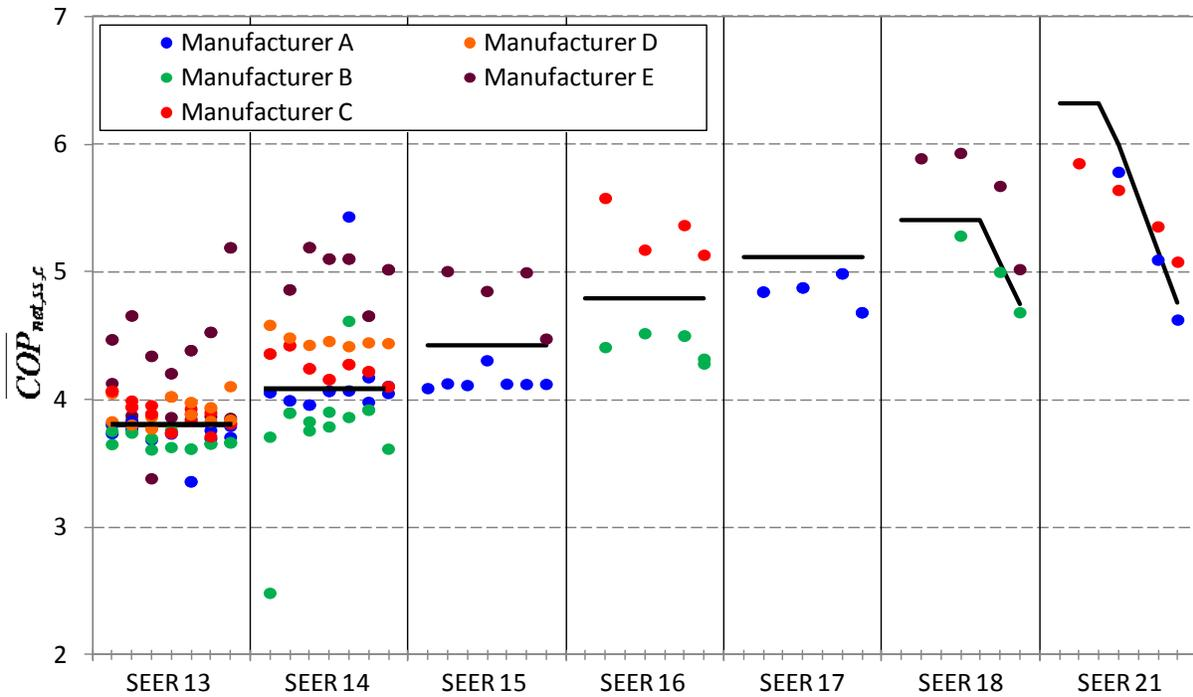
**Figure 10. Simulation results for the AC library (shown in solid black lines) compared to individual AC units (individual capacities of 1.5, 2, 3, 4, and 5 tons shown in ascending order within SEER values)**
