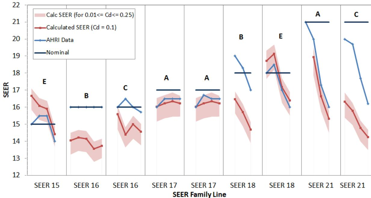
**Figure 9. SEER calculated using manufacturer data compared to AHRI reported SEER values for two-stage ACs (letters A, B, C, and E denote manufacturer; capacities of 2, 3, 4, and 5 tons shown in ascending order within a product line)**
