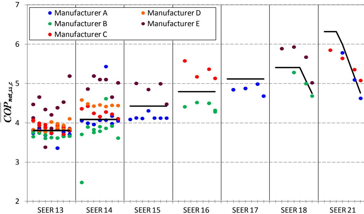
**Figure ES–1. Simulation results comparing annual average efficiency of a standard AC component library (shown in black lines) to specific AC units for five leading manufacturers (1.5-, 2-, 2.5-, 3-, 3.5-, 4-, and 5-ton sizes shown for each SEER family, when available)**
