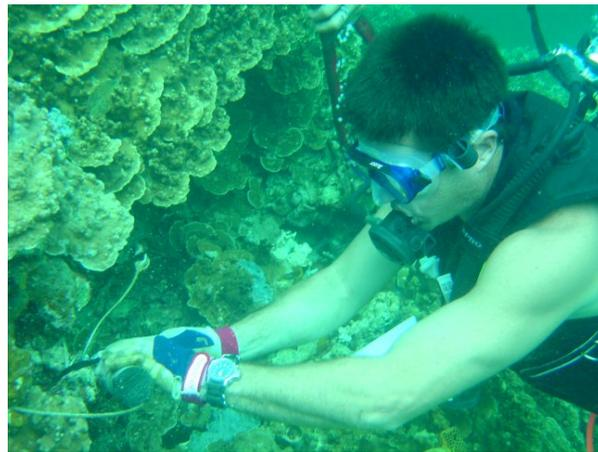
**Figure 5 Cary McLean secures an SBE39 temperature logger to a coral outcrop using stainless steel wire.**
