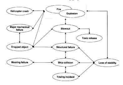
A key element of risk management is a structured hazard identification and control process. The Guidelines recommend that this process be based upon international standards (ISO 17776). The following diagram provides an example representation of a hazard scenario evaluation, with the identification of the associated risk management barriers.
