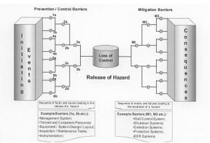
Having been so identified, the barriers can then be assessed for their criticality and effectiveness, responsibility assigned for their maintenance, and arrangements made for their verification, as appropriate. It can be appreciated that in a complex facility, such as an operating MODU, there will be thousands of barriers identified.
