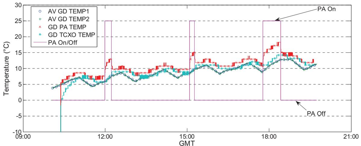
Figure 4.—Temperature increase when the SDR is transmitting (November 2, 2012).
