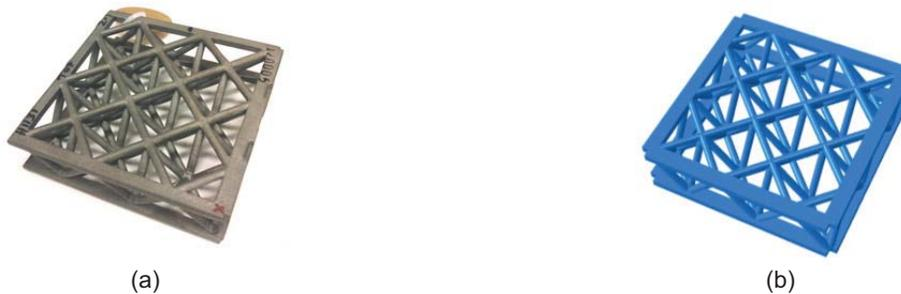
Figure 24.—(a) SMA lattice casting, and (b) Abaqus finite element model.
