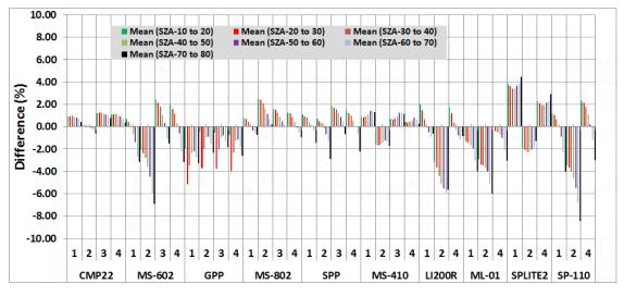
Figure 3: Mean percent differences for six thermopile pyranometers (first six) and four photodiode pyranometers (last four).
