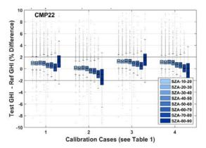
**Figure 1:** Indoor and outdoor calibration comparison of the reference GHI irradiance to the CMP22 test radiometer irradiance.
