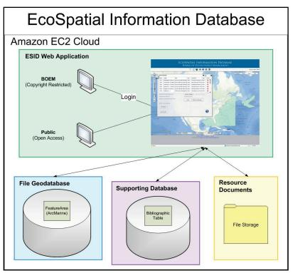
Figure 29. Components of the ESID Web Application.
