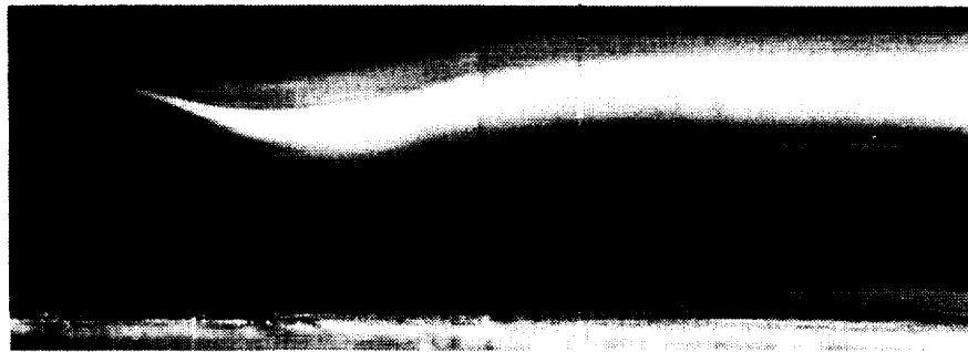
Figure 21 Photograph of flow visualization without suction, grid 0, Re = 50,000
