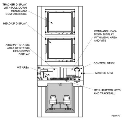
**Figure 2. Pilot rack setup with heads-up display and tracker display**. (*Reprinted from* Air Force Technical Order (TO) 1Q-9(M) A-1, *Flight Manual, USAF Series MQ-9 Aircraft*, change 1, 2 May 2014, 1-79.)
