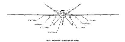
**Figure 3. MQ-9 station depiction**. (*Reprinted from* TO 1Q-9(M) A-34-1-1, *Technical Manual, USAF Series MQ-9 Aircraft Nonnuclear Munitions Delivery*, change 1, 1 March 2014, 1–3.)
