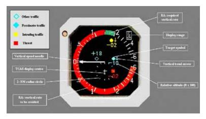
**Figure 1.TCAS RA display implemented on an instantaneous vertical speed indicator**. (*Reprinted from* FAA, "Introduction to TCAS II," version 7.1, 28 February 2011, 15.)
