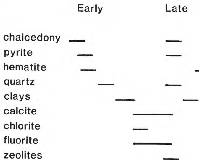
FIGURE 21.—Generalized paragenetic sequence of principal hydrothermal minerals in drill core Y-3. Length of lines is not indicative of duration of mineral deposition.
