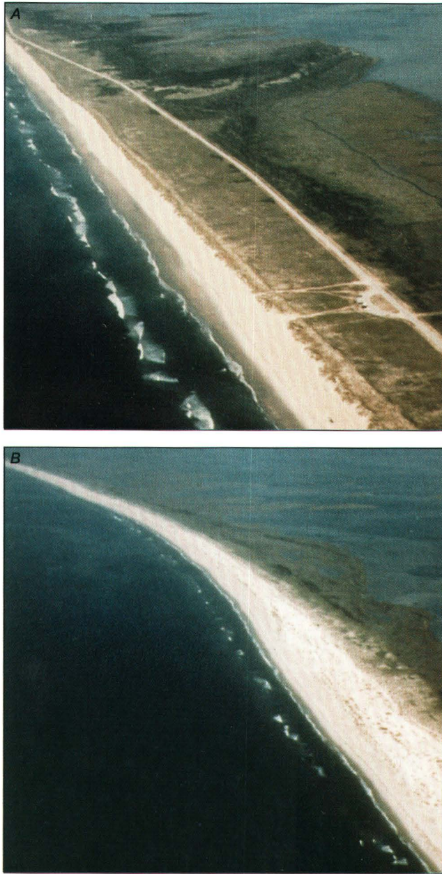
Figure 59. The difference in beach widths can be seen from these two photographs. A, Hatteras Island (stabilized), and B, Core Banks (unstabilized). (Source: R. Dolan.)
