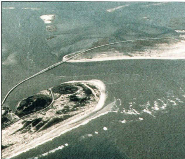
Figure 28. Pattern of sedimentation at Oregon Inlet. (Source: R. Dolan.)
