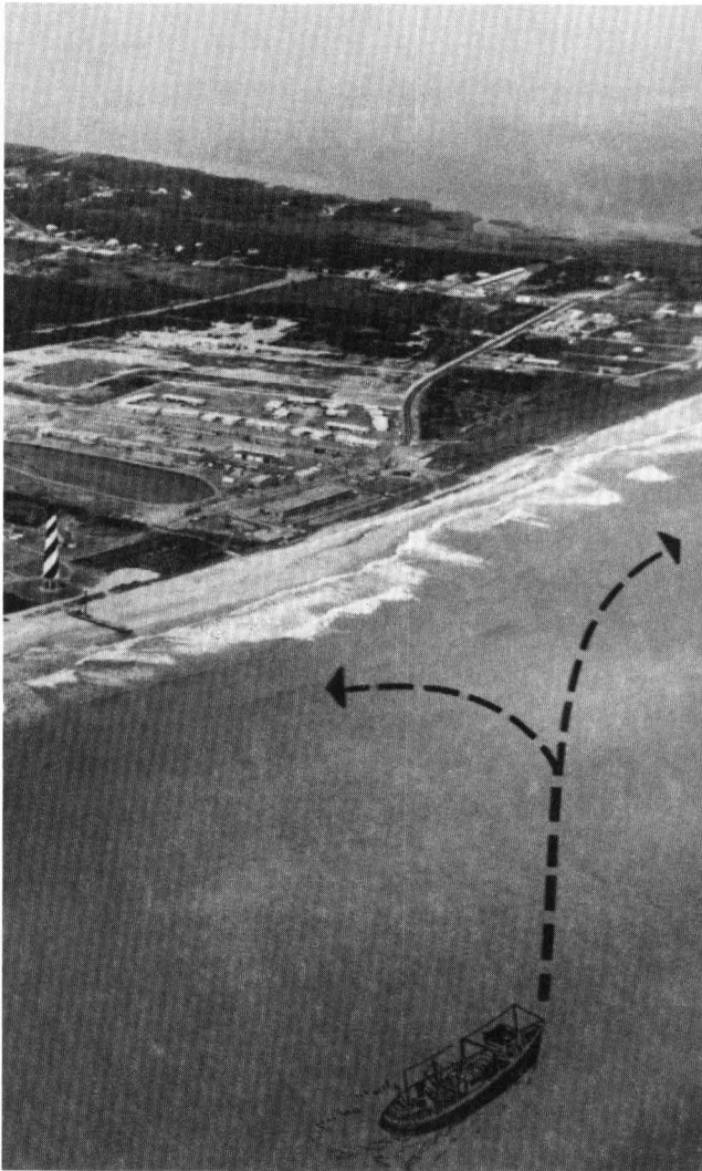
Figure 53. The concept of transferring sand from offshore shoals to the inshore zone near Cape Hatteras. (Source: R. Dolan.)
