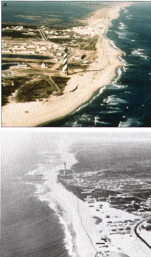
Figure 51. Cape Hatteras. A, Groins trap sand that normally moves along the shoreline, 1971, and B, Beach nourishment, 1974. (Source: R. Dolan.)
