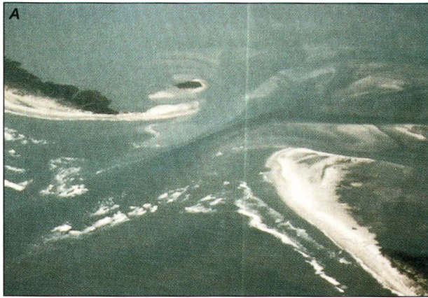
Figure 12. Features of inlet sedimentation. New lands are created as tidal deltas become vegetated. A, Floodtide delta in upper right of photograph, ebbtide delta in lower left. B, Diagram of inlet features. C, Inlet features following inlet closure. (Source: J. Fisher.)
