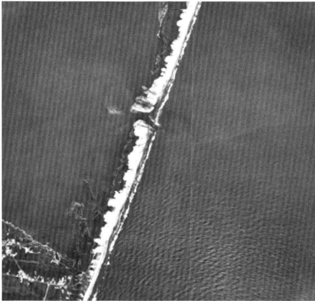
Figure 32. Pattern of storm-surge penetration along Hatteras Island, 1962. (Source: U.S. Army.)
