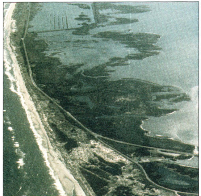
Figure 13. The pattern of clearly evident oceanic overwash and inlet sedimentation on the bay side of Pea Island. (Source: R. Dolan.)
