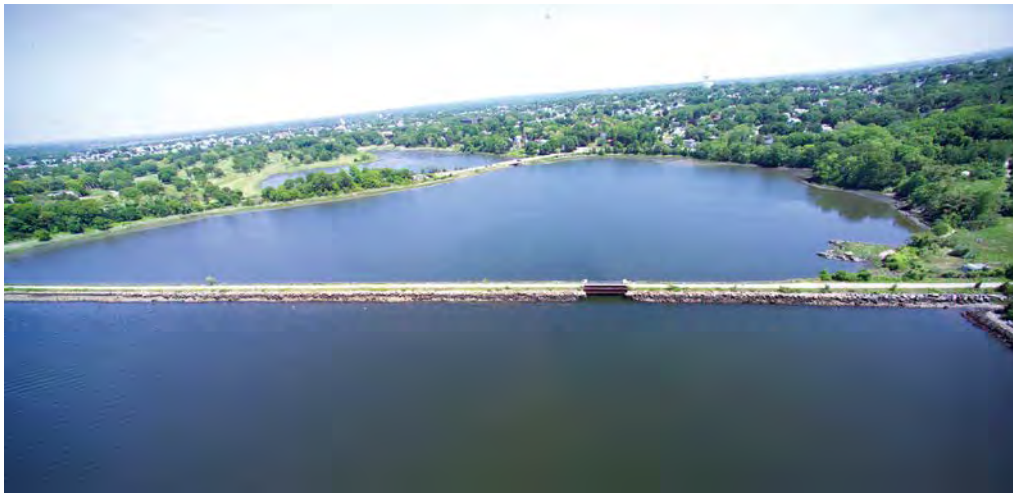
Figure 4-4. Hydrological evidence for poor connectance—Watchemocket Cove, RI, is connected to Narragansett Bay only under a small bridge on an old railroad causeway.
