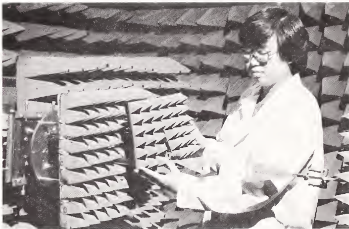
Douglas T. Tamura, an electronics technician, aligns antennas being calibrated on the extrapolation range, which is part of the near-field antenna measurement facility.
