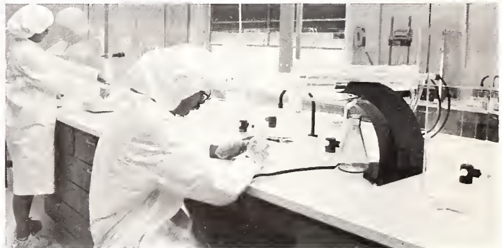
The NIST ultra-clean ceramic processing laboratory is specially designed for the production and processing of advanced ceramic powders and samples with controlled levels of impurities and dopants.
