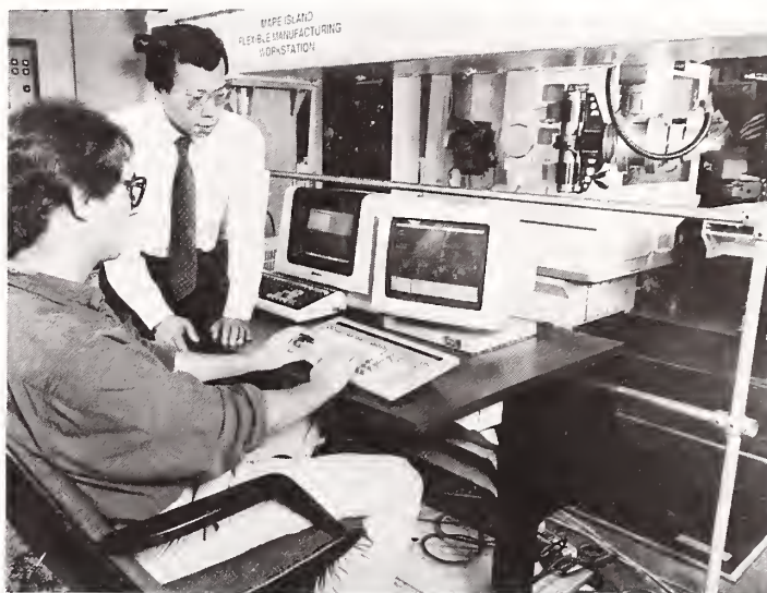
Electronics technician Michael Huff (left) and project chief Kang Lee monitor the Mare Island Flexible Workstation, the first large-scale transfer of flexible and automation technology from the AMRF to a production facility.
