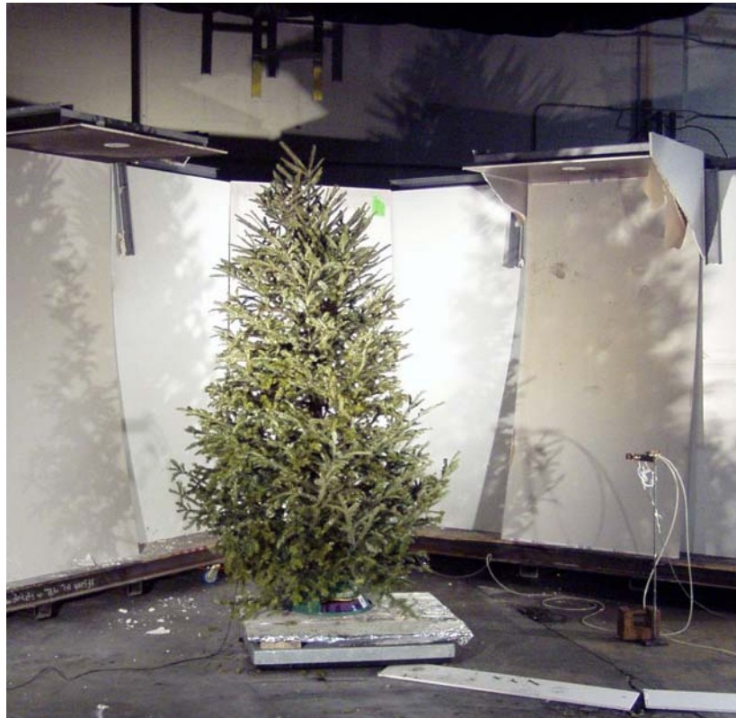
Figure 2. Tree in stand on load cell under oxygen consumption calorimetry hood
