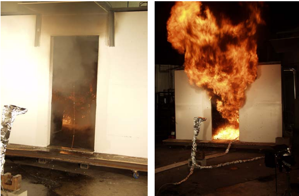
Figure 17. Comparison of the sprinklered room, on the left, with the unsprinklered room (Both photos were taken at approximately 1 minute after ignition.)
